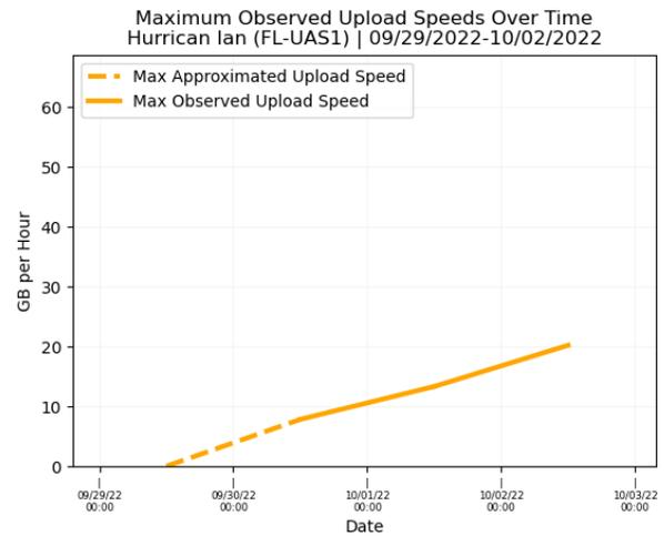
Fig. 7. Maximum observed upload rate at the FOB at each date in the response in GB/hr. On 9/29 no observations of wireless upload speeds were made from which a maximum could be computed. The upload rate on that date has been approximated as 0 GB/hr and plotted it here as a dashed line for awareness.
