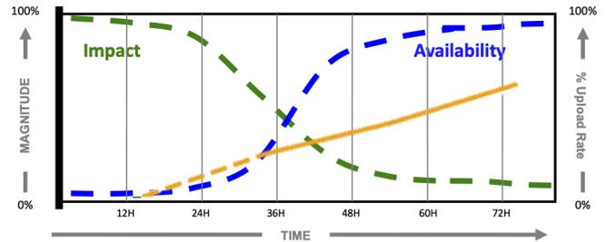
Fig. 2. Impact (green dashed) versus availability of information (blue dashed) to emergency responders during the first 72 hours of a disaster, adapted from [3]. Scaled availability of drone data products as % update rate over wireless networks at Hurricane Ian in gold.
