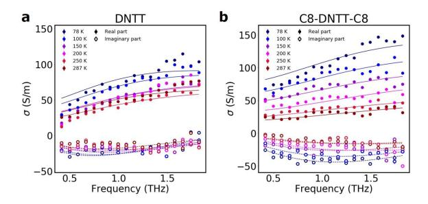
**Figure 3:** Frequency dependent THz photoconductivity. The data refer to 0.5 ps after 3.1 eV excitation of (a) DNTT and (b) C8-DNTT-C8 samples. The lines are fitting to the Drude-Anderson model described in the text (solid lines indicate the real part, and the dashed line the imaginary part of the conductivity).
