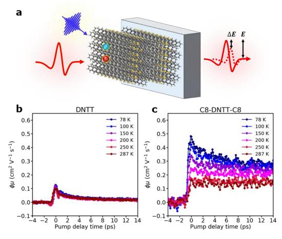
**Figure 2:** *T*-dependent photoconductivity studies by optical-pump THz-probe (OPTP) spectroscopy in DNTT and C8-DNTT-C8. (a) Schematic illustration of the OPTP spectroscopy. Photoconductivity dynamics of (b) DNTT and (c) C8-DNTT-C8 as a function of temperature with 3.1 eV excitation.
