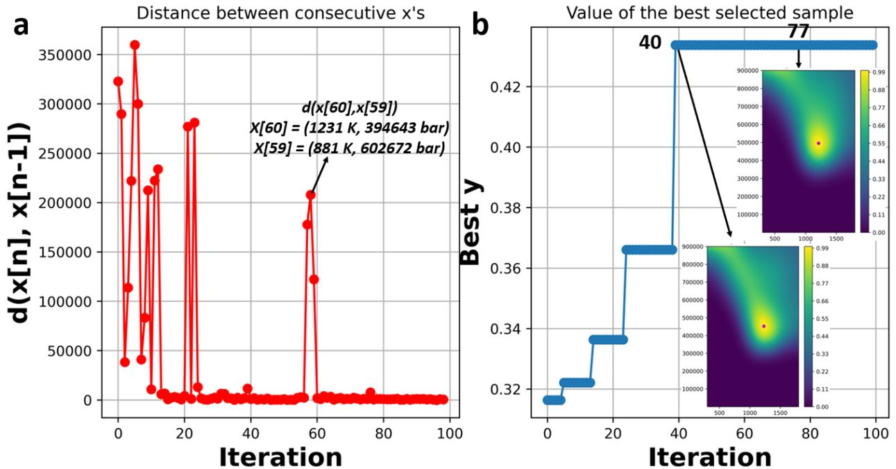
**Figure 7. (a)** The changes of distance between consecutive points suggested by the acquisition function corresponding to the iterations  $n$  and  $n-1$  with iteration number **(b)** The changes of best observation calculated using the MD simulation with the iteration number. Two subfigures show the acquisition function distribution for iterations 40 and 77.  $\sigma_y$  and  $\delta$  are equal to 0.03 and 0.01 for the BO task.
