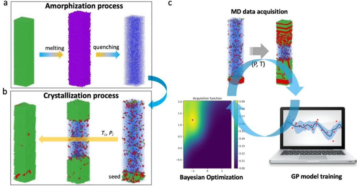
**Figure 1.** (a) Amorphization of fcc-Ni and (b) crystallization of a-Ni. The green, purple, blue and red particles show atoms with fcc, melt, amorphous and hcp phases, respectively. (c) Flowchart of the BO process that iterates between MD data acquisition, GP model training and BO prediction.
