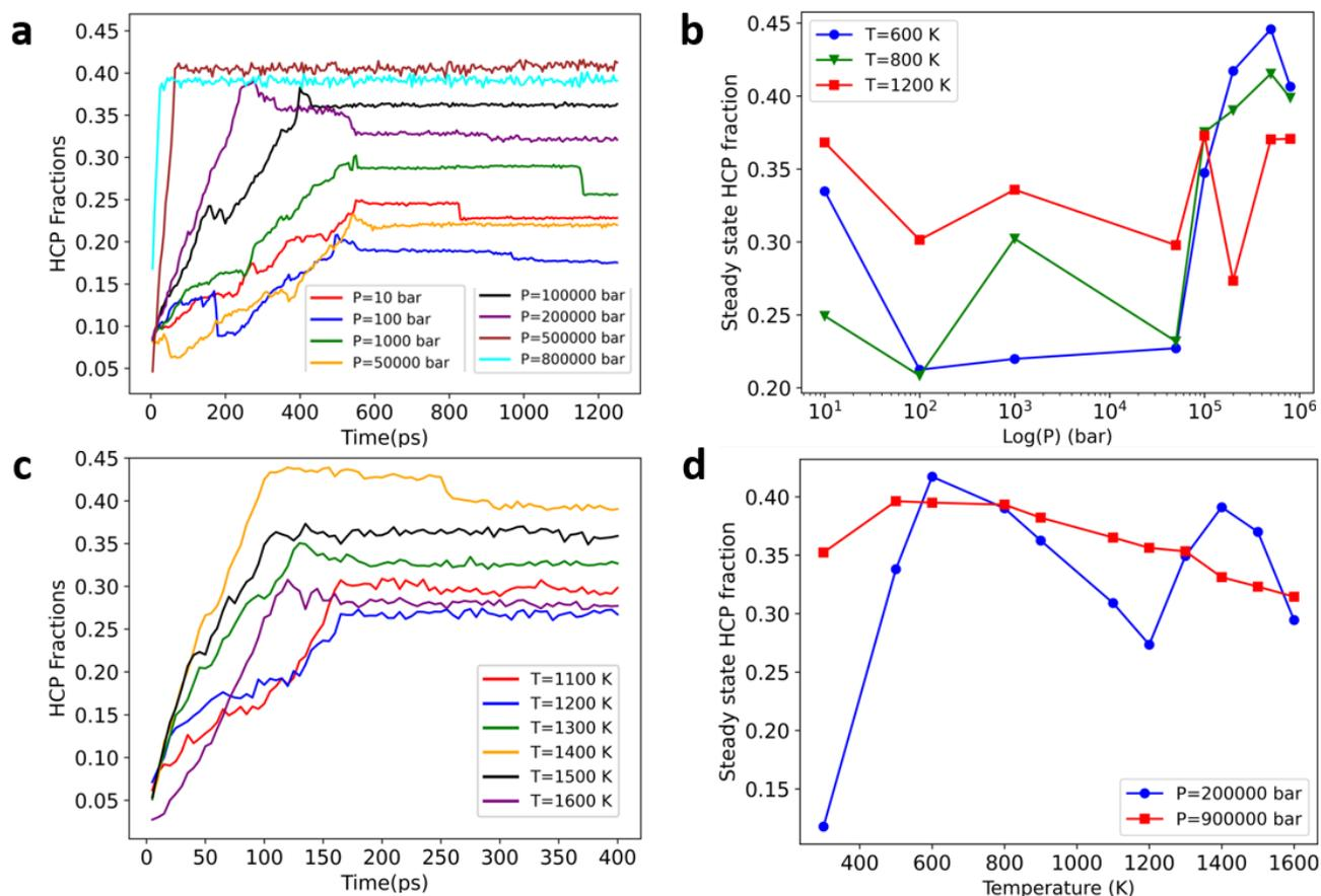
**Figure 2.** (a) Fractions of hcp-Ni phase as a function of time for crystallization of a-Ni with a hcp seed at 800 K and different pressures. (b) The steady-state hcp-Ni fraction at different temperatures as a function of logarithmic pressure. (c) Fractions of hcp-Ni versus time at 200,000 bar and different temperatures. (d) The steady-state hcp-Ni fraction at different pressures as a function of temperature.
