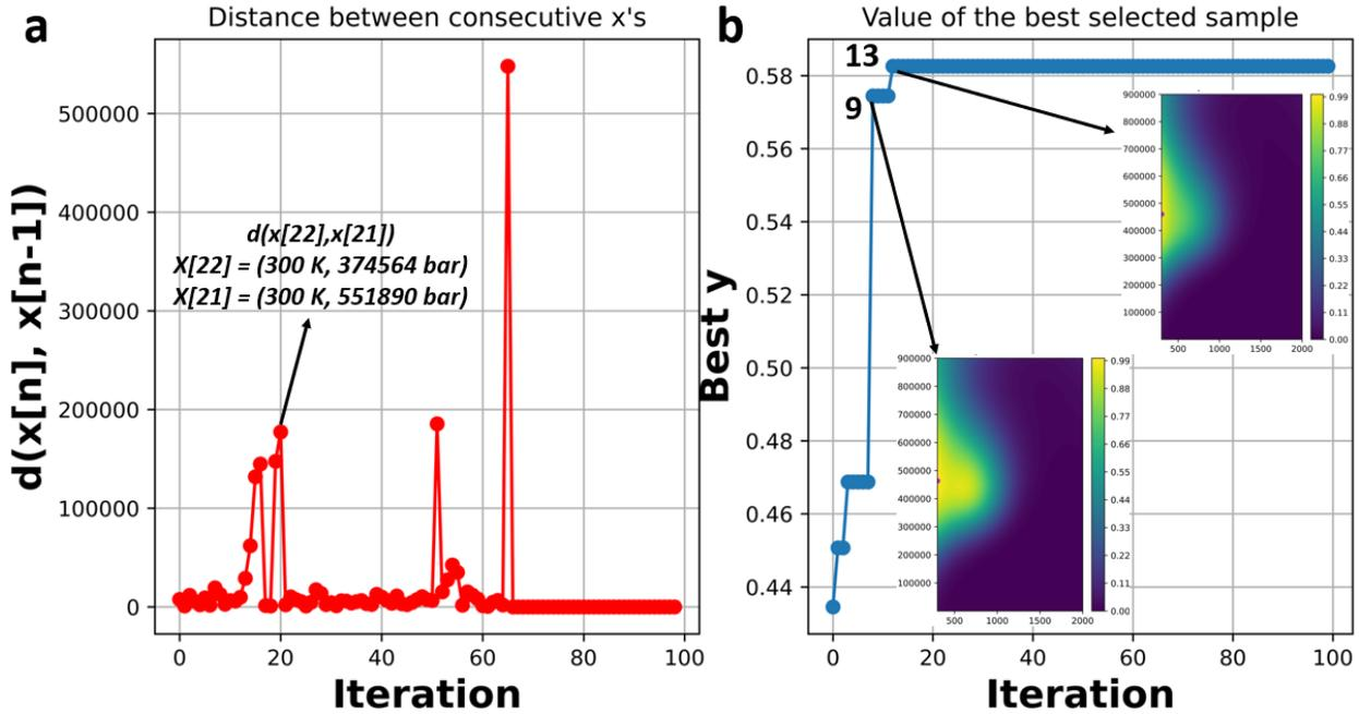
**Figure 5.** (a) The changes of distance between consecutive points suggested by the acquisition function corresponding to the iterations  $n$  and  $n-1$  with iteration number (b) The changes of best observation calculated using the MD simulation with the iteration number. Two subfigures show the acquisition function distribution for iterations 9 and 13.  $\sigma_y$  and  $\delta$  are equal to 0.1 and 0.01 for the BO task.
