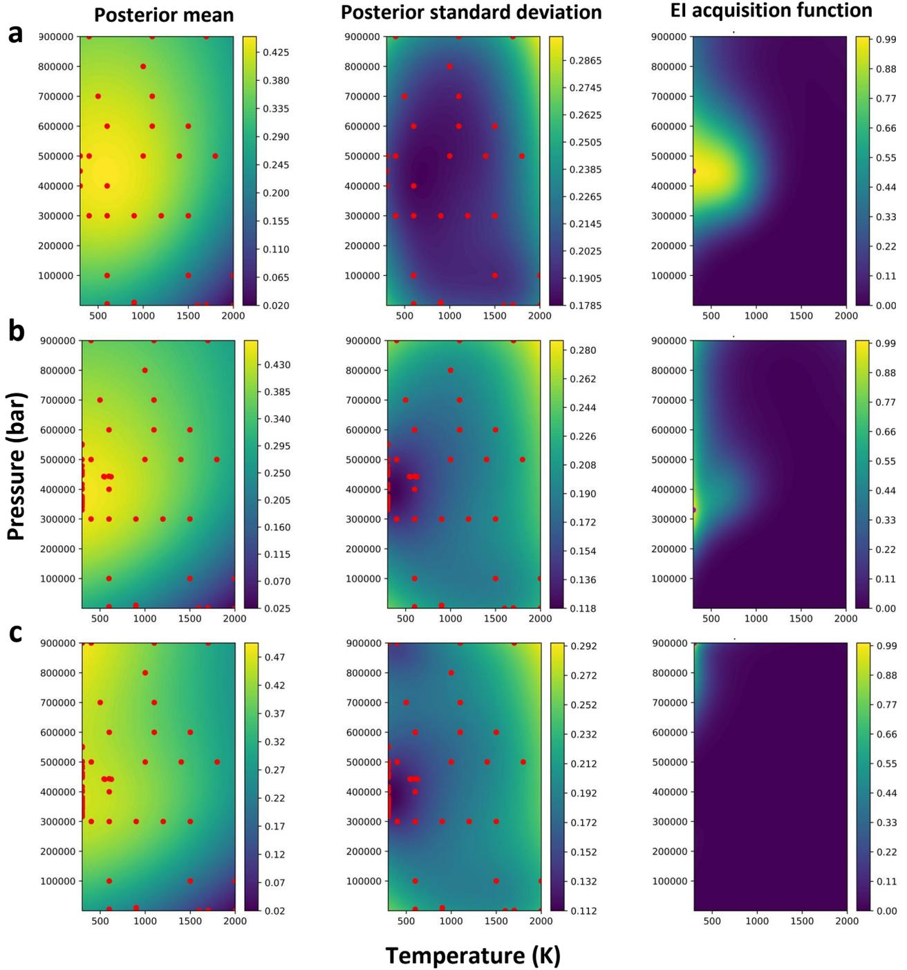
**Figure 4.** Posterior mean, posterior standard deviation and normalized EI acquisition function for the BO of hcp-Ni fraction from crystallization with an hcp seed for iterations (a) 1, (b) 50, and (c) 85.
