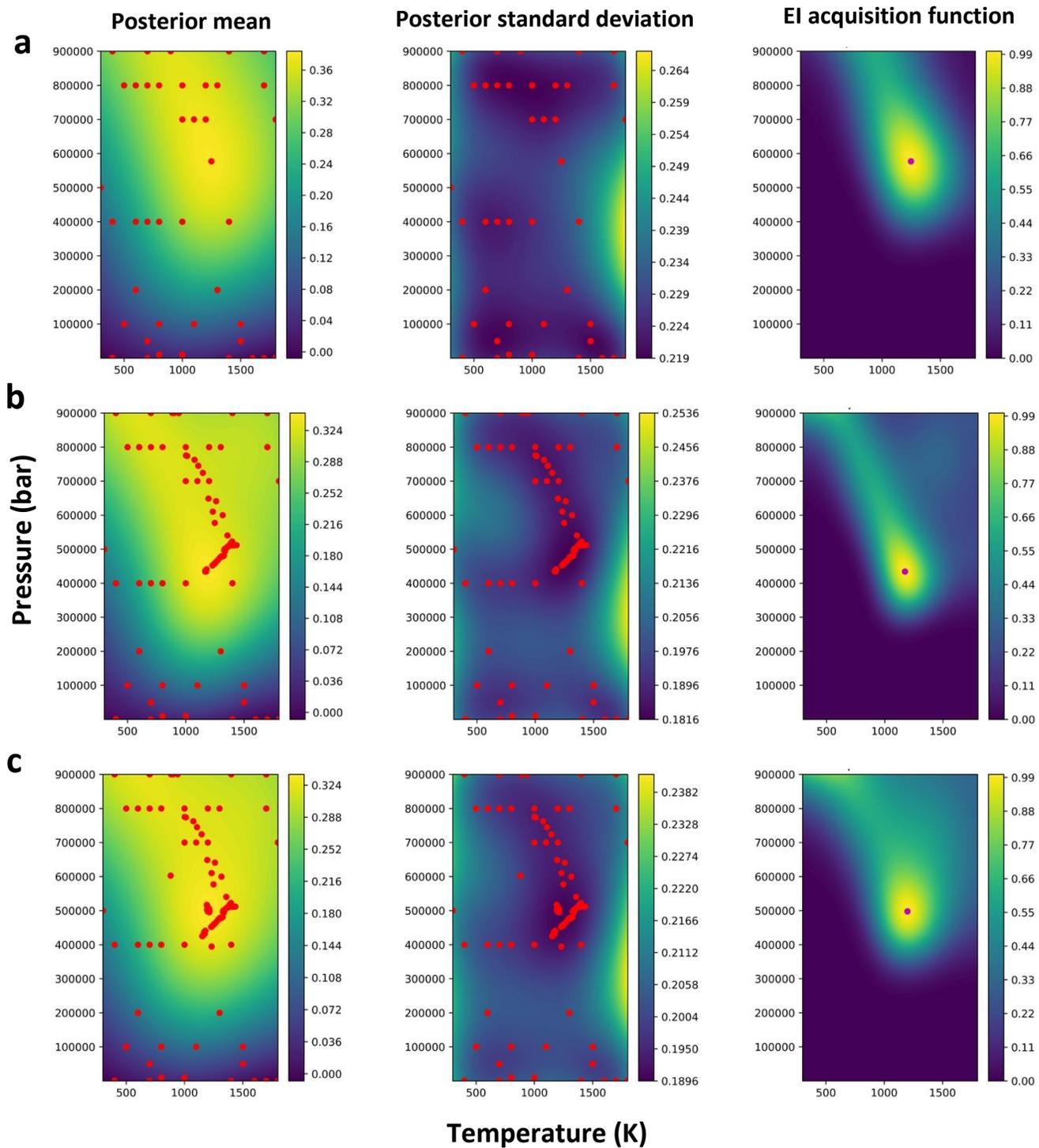
**Figure 6.** Posterior mean, posterior standard deviation and normalized EI acquisition function for the BO of hcp-Ni fraction from crystallization with an fcc seed for iterations (a) 1, (b) 50, and (c) 85.
