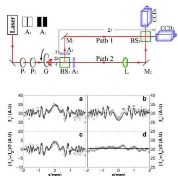
Fig. 5-6 Experimental data of intensity distributions (circles). (a) and (b) are the interference patterns registered by CCD<sub>1</sub> and CCD<sub>2</sub>, respectively; (c) and (d) are their difference and summation, respectively (Gan et al., 2009).
