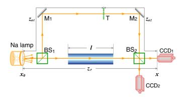
Fig. 4-9 An equal-optical-path interferometer, where a glass rod of length l is placed in one arm, and T is an object in the other arm. The interferometer is illuminated by a sodium lamp. (Zhang et al., 2009b)
