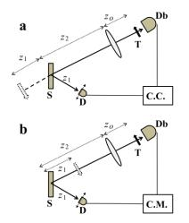
Fig. 3-9 Sketches of ghost imaging: S, source; T, object; Db, bucket detector; D, scanning detector; C.C., coincidence counting; C.M., correlation measurement. (a) S is a two-photon entangled source, which acts as a mirror; (b) S is a thermal light source, which acts as a phase-conjugation mirror.
