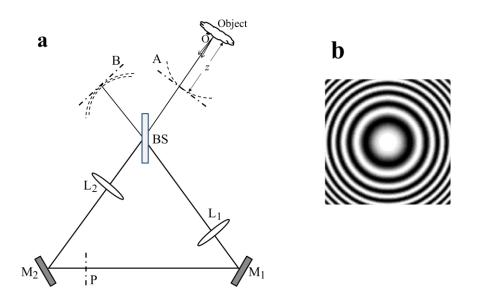
Fig. 2-1 (a) Sketch of a triangular interferometer. BS is a beamsplitter,  $M_1$  and  $M_2$  are two mirrors,  $L_1$  and  $L_2$  are two lenses with their focal planes located at A and B, respectively. (b) Fresnel zone plate (FZP) pattern.
