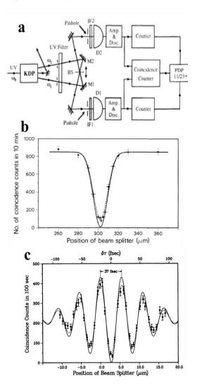
Fig. 3-4(a) Experimental setup of Hong-Ou-Mandel interferometer; (b) Experimental result for the degenerate two-photon state. The measured number of coincidences as a function of beam-splitter displacement (Hong et al., 1987). (c) Experimental result for the non-degenerate two-photon entangled state (Ou and Mandel, 1988).
