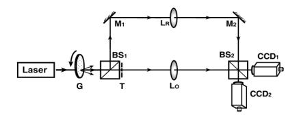
Fig. 4-4 Unequal-optical-path interferometer with lenses, which are inserted in the centre of the two arms. Both the input and output ports of the interferometer are located at the two focal planes of the lenses (Gao et al., 2009).
