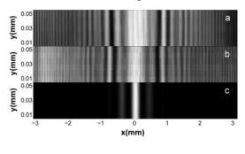
Fig. 4-8 Experimentally observed 2D interference patterns registered by  $CCD_1$  in the scheme of Fig. 4-6: (a) with the pseudo-thermal light source, averaged over 10000 frames; (b) with a Na lamp of extended illumination area as the light source; (c) with a Na lamp followed by a pinhole as the light source (Zhang et al., 2009a).
