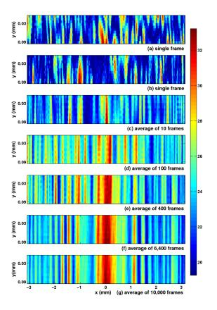
Fig. 4-2 Experimentally observed 2D interference patterns recorded by CCD<sub>1</sub>. (a) and (b) are individual single frames; (c), (d), (e), (f) and (g) are averaged over 10, 40, 400, 6400 and 10000 frames, respectively. The color-bar shows the relative intensity (Zhang et al., 2010a).
