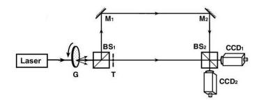
Fig. 4-1 Experimental scheme for an unequal-optical-path interferometer where the two arms have different lengths. A laser and a rotating ground glass disk G form a spatially incoherent source;  $M_1$  and  $M_2$  are mirrors,  $BS_1$  and  $BS_2$  are beamsplitters,  $CCD_1$  and  $CCD_2$  are detectors, and T is a double-slit close to  $BS_1$  (Zhang et al., 2009a).
