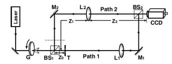
Fig. 4-12 Experimental setup of ghost imaging in first-order interference (Gao et al., 2009b).
