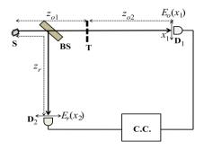
Fig. 3-8 Sketch of ghost diffraction: S, source; BS, beamsplitter; T, object;  $D_1$  and  $D_2$ , two detectors; C.C., coincidence counting measurement.
