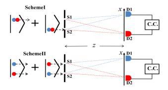
Fig. 3-3 Two types of two-photon entangled states partaking in second-order interference.
