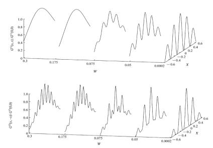
Fig. 3-7 The first-order (above) and second-order (below) double-slit interference patterns when the normalized spatial spectrum width *W* is varied (Wang et al., 2006).
