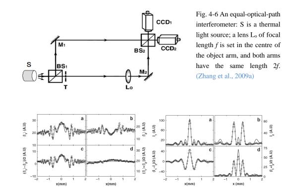
Fig. 4-7 Experimentally observed 1D interference patterns in the scheme of Fig. 4-6. Left and right parts are the patterns using spatially incoherent and coherent light, respectively. (a) and (b) are interference patterns (averaged over 10000 frames for the incoherent case) registered by CCD1 and CCD2, while (c) and (d) are their difference and summation, respectively. Experimental data are given by open circles and theoretical simulation by solid lines (Zhang et al., 2009a).
