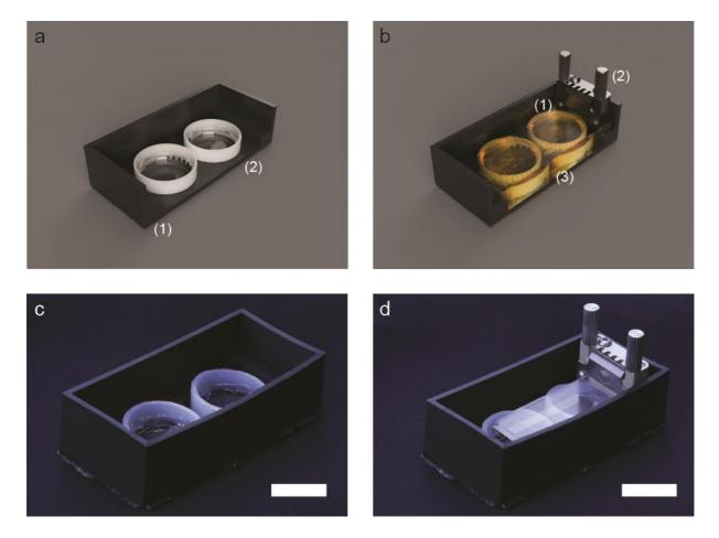
**Figure S5.** 3D printed emulsion container used to manufacture the active shutter elements. (a) Rendering of the (1) 3D printed container showing (2) two PTFE tubes partially filled with poly(dimethylsiloxane) (PDMS, Sylgard 184, Dow Corning). (b) Rendering of the printed holder with (1) the microfluidic device attached to (2) the Dolomite connector immersed in (3) the monomer mixture. (c-d) Photographs of the actual container alone and with the microfluidic device. Scale bar is 2 cm.
