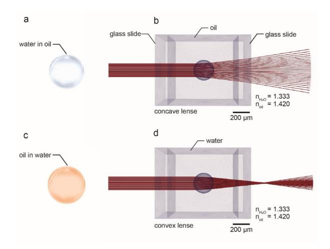
**Figure S4.** (a-b) Ray trajectories ( $\lambda = 532 \text{ nm}$ ) for a water droplet with index of  $n_{H_2O} = 1.333$  in oil ( $n_{oil} = 1.420$ ). The microlens acts as a concave lens with negative focal length and negative focal power. (c-d) Ray trajectories ( $\lambda = 532 \text{ nm}$ ) for an oil droplet with index of  $n_{oil} = 1.42$  in water  $n_{H_2O} = 1.333$ . The microlens acts as a convex lens with positive focal length and positive focal power.
