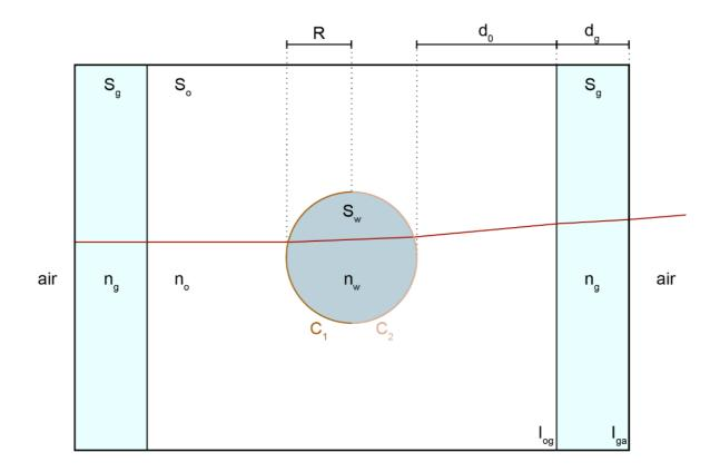
**Figure S2.** Schematic illustrating the different optical elements used for the analytical ray tracing model, including two glass slides  $(S_g)$  of refractive index  $n_g$ , the oil domain  $(S_o)$  with refractive index  $n_o$  and the water droplet  $(S_w)$  with refractive index  $n_w$ . The interfaces between the optical elements are indicated by  $C_1$ ,  $C_2$ ,  $I_{og}$  and  $I_{ga}$ . R,  $d_o$  and  $d_g$  represent the lengths and distances from the experimental system.
