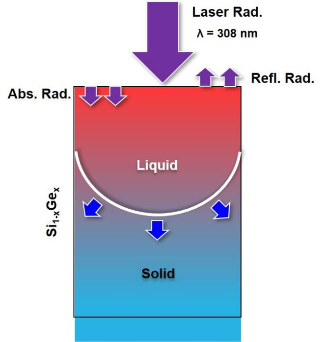
**Figure 1:** Schematics of the laser-melting process with laser radiation (Laser Rad.), absorbed radiation (Abs. Rad.) and reflected radiation (Refl. Rad.). Warmer areas are red-coloured, colder ones blue-coloured.
