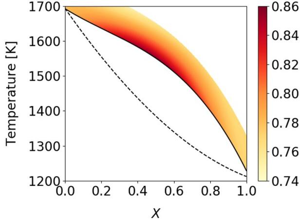
**Figure 5:** Reflectivity map of liquid  $Si_{1-x}Ge_x$  at a wavelength of 308 nm as a function of temperature and alloy fraction. The continuous line represents the liquidus and the dashed one the solidus thermodynamic limits, redrawn from Olesinski and Abbaschian (1984).
