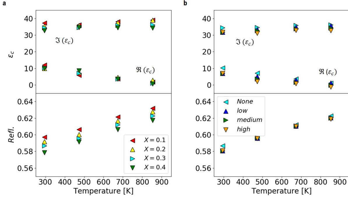
**Figure 2:** Imaginary,  $\Im(\epsilon_c)$ , real,  $\Re(\epsilon_c)$  parts of dielectric functions values and associated reflectivities measured at 308 nm by spectroscopic ellipsometry at different temperatures and alloy fractions for undoped  $Si_{1-x}Ge_x$  (a), and  $X=0.3$  boron doped  $Si_{1-x}Ge_x$  samples (b).
