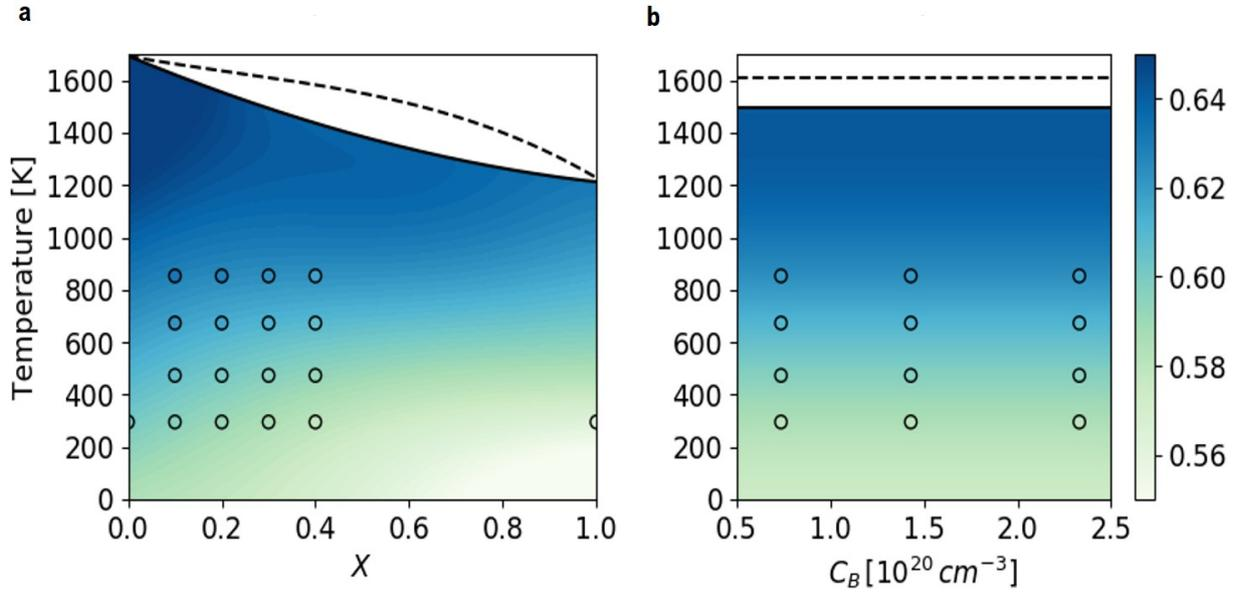
**Figure 3:** Reflectivity of  $Si_{1-x}Ge_x$  obtained from fitted  $\epsilon_c$  for undoped (a) an p-doped  $X=0.3$  samples (b). The continuous line represents the solidus thermodynamic limit and the dashed one the liquidus, redrawn from Olesinski and Abbaschian (1984). Coloured dots represent the experimental values.
