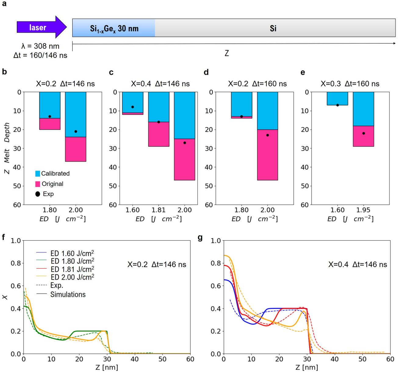
**Figure 6:** Schematics of the mono-dimensional model employed for laser annealing simulations on strained  $Si_{1-x}Ge_x$  samples (a), comparison between experimental and simulated MDs for a laser pulse of 146 ns (b)(c) and 160 ns (d)(e), experimental vs simulated germanium profile for  $X=0.2$  (f) and  $X=0.4$  (g) with  $\Delta t$  of 146 ns, the experimental profiles are re-drawn from Dagault et al. (2019, 2020). Cf. main text for definitions of original and calibrated models.
