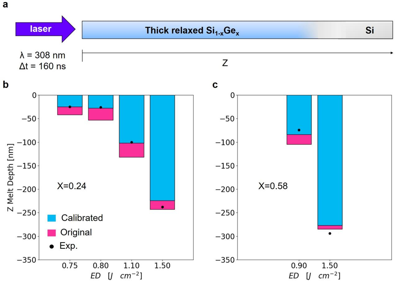
**Figure 4:** Schematics of the mono-dimensional model employed for simulating laser annealing on relaxed  $Si_{1-x}Ge_x$  samples (a), comparison between experimental and simulated MD for relaxed  $Si_{1-x}Ge_x$  samples with initial alloy fractions of 0.24 (b) and 0.58 (c). Cf. main text for definition of calibrated and original models
