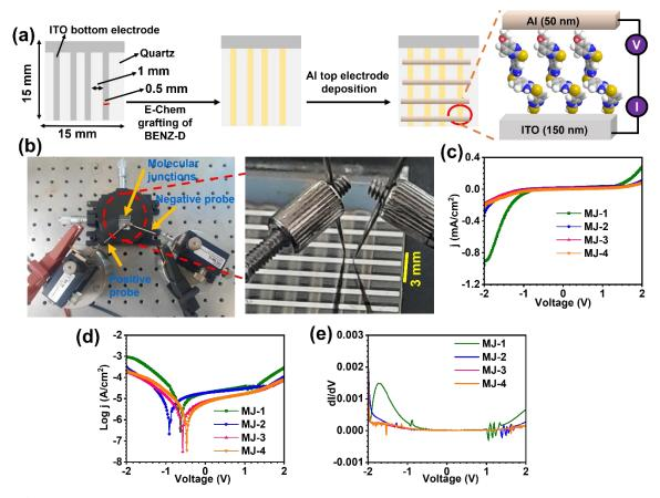
**Figure 4.** (a) Fabrication of ITO/BENZ/Al molecular electronic devices, (b) electrical measurements set-up, (c) j-V plot, (d) log j-V and (e) dI/dV vs V plots of MJ-1 to MJ-4.
