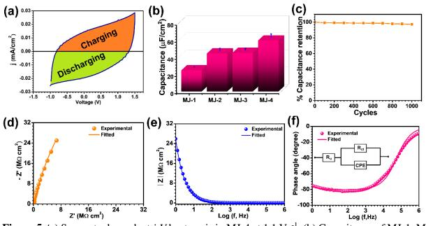
**Figure 5.** (a) Scan rate dependent *j*-*V* hysteresis in MJ-4 at 1 1 Vs<sup>-1</sup>, (b) Capacitance of MJ-1, MJ-2, MJ-3 and Mj-4 at 10 mVs<sup>-1</sup>, (c) capacitance retention in MJ-4 up to 1000 cycles, (d) Nyquist plot, (e)&(f) Bode plot of MJ-4 at V= 0 DC voltage in the frequency range  $10^6$  to 1 Hz with 100 mV amplitude.
