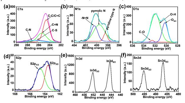
**Figure 3.** High-resolution and deconvoluted XPS spectra of (a) C1s, (b) N1s (c) O1s, (d) S2p, (e) In3d and (f) Sn3d of Films-4.
