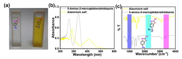
**Figure 1.** (a) Digital photograph of solutions of 5-amino-2-mercaptobenzimidazole (left) and diazonium salt (right), (b) comparison of UV-vis spectra and (c) comparison of FT-IR spectra of 5-amino-2-mercaptobenzimidazole (gray) and diazonium salt (yellow).
