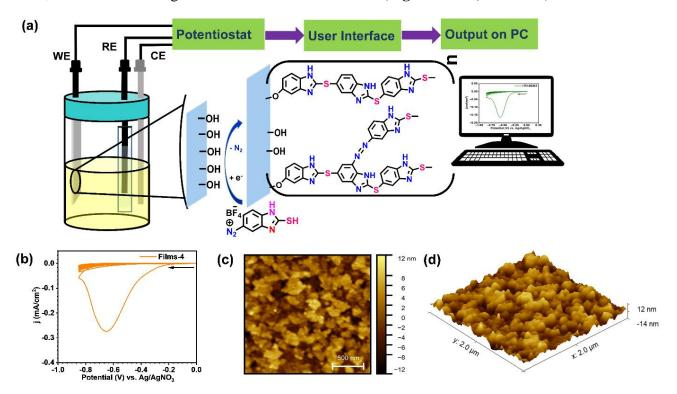
**Figure 2.** (a) The three-electrode electrochemical system for the reduction of BENZ-D, (b) cyclic voltammogram of E-Chem grafting of BENZ molecular layers on ITO electrodes (Films-4) and (c-d) 2 D and 3D AFM image of Films-4.
