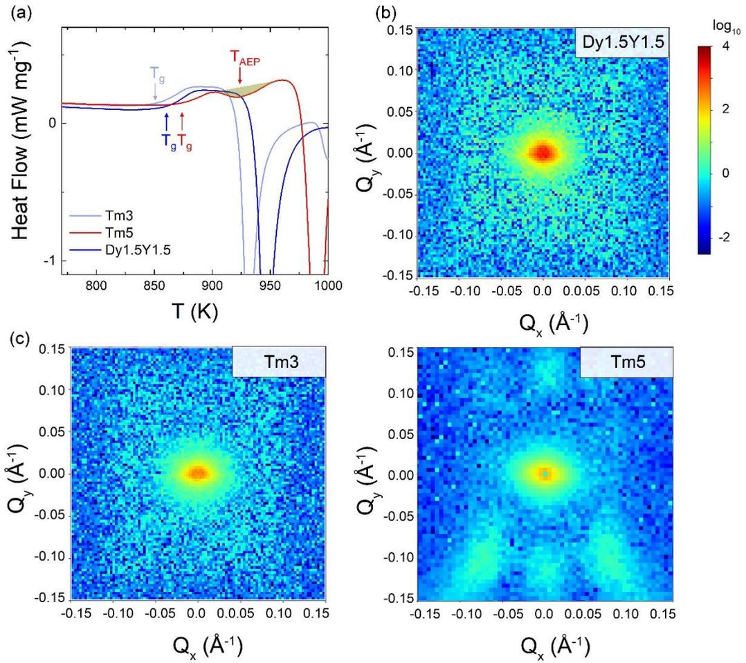
**Fig. 7** DSC curves for  $(\text{Fe}_{0.73}(\text{Dy}_{0.5}\text{Y}_{0.5})_{0.03}\text{B}_{0.24})_{96}\text{Nb}_4$  (abbreviated Dy1.5Y1.5),  $(\text{Fe}_{0.73}\text{Tm}_{0.03}\text{B}_{0.24})_{96}\text{Nb}_4$  (abbreviated Tm3) and  $(\text{Fe}_{0.71}\text{Tm}_{0.05}\text{B}_{0.24})_{96}\text{Nb}_4$  (abbreviated Tm5) MGs. 2D total scattering cross section for (b) Dy1.5Y1.5 (c) Tm3 and (d) Tm5 with an applied magnetic field of 0.05 T.
