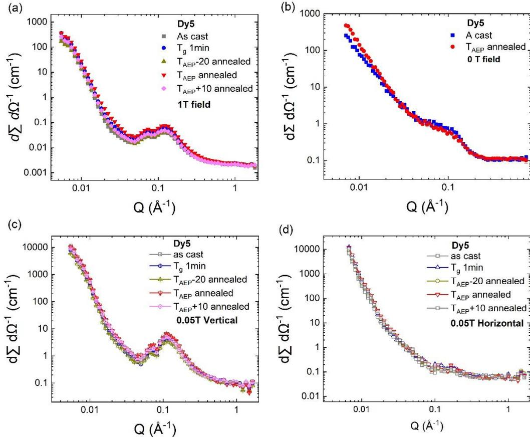
**Fig. 5.** (a)  $d\Sigma/d\Omega$  for Dy5 in different states at 1 T field. (b)  $d\Sigma/d\Omega$  for Dy5 in as-cast state and  $T_{AEP}$ -annealed state with no magnetic field. (c) Magnetic azimuthally averaged SANS cross sections in the vertical direction, and (d) magnetic azimuthally averaged SANS cross sections in the horizontal direction under an applied magnetic field of 0.05 T.
