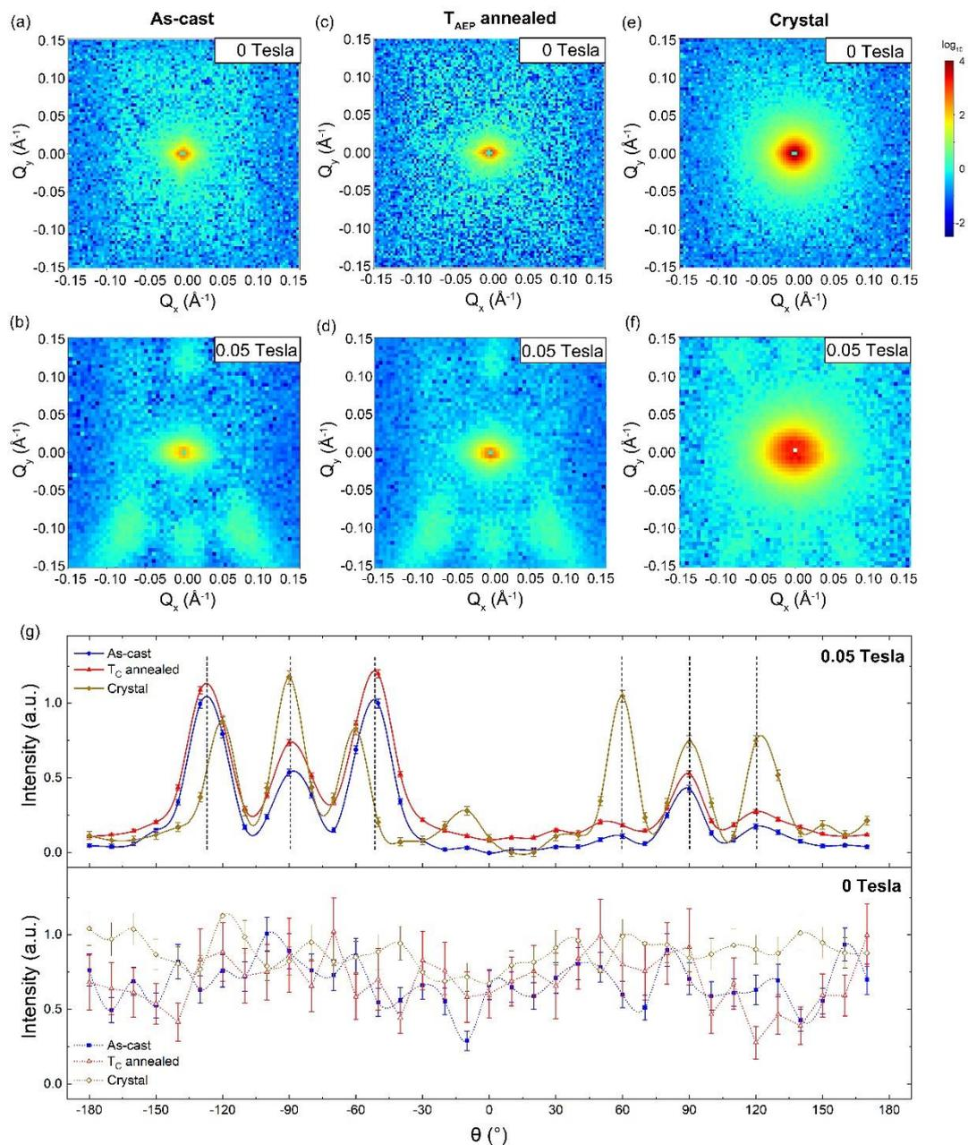
**Fig. 6** 2D total scattering SANS cross section for (a) as-cast, (c)  $T_{\text{AEP}}$ -annealed, and (e) crystal Dy5 under zero magnetic field with a reduced  $Q$  range. 2D total scattering SANS cross section for (b) as-cast, (d)  $T_{\text{AEP}}$ -annealed, and (f) crystal Dy5 under 0.05 field (measured at CSNS). (g) Normalized intensity under 0.05 T (upper) and 0 T (lower) at
