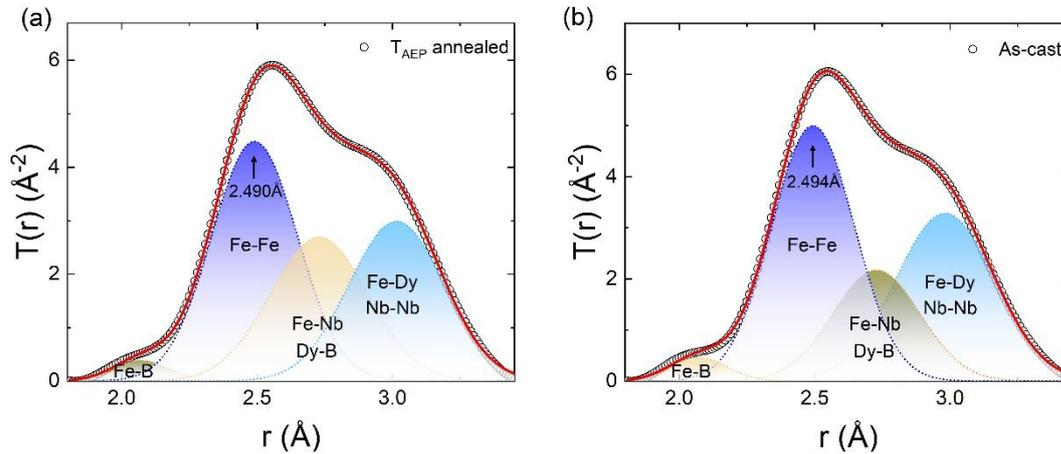
**Fig. S6** Fit of a linear combination of Gaussians to first-shell peaks of x-ray  $T(r)$ , obtained by  $4\pi\rho_0r + G(r)$ , where  $\rho_0$  is the number density. (a) Fit of  $T_{\text{C}}$ -annealed Dy5
