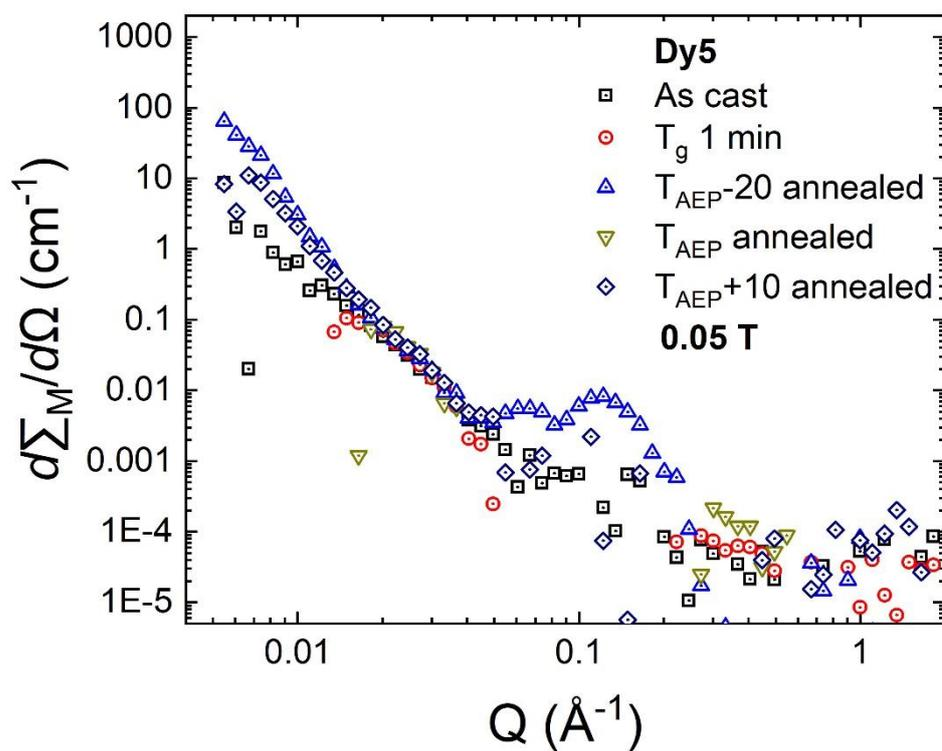
**Fig. S4** Magnetic spin-misalignment SANS cross sections under 0.05 T magnetic field, obtained by subtracting the scattering cross section  $d\Sigma/d\Omega$  at a saturating magnetic field of 1 T from the scattering cross section at 0.05 T.
