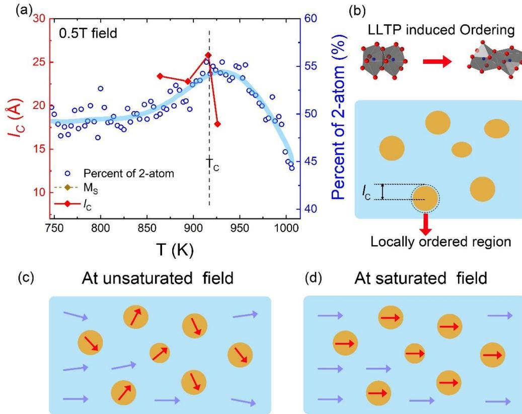
**Fig. 8.** (a) Evolution of 2-atom cluster connectivity, saturation magnetization, magnetic correlation length, and intraparticle correlation length as a function of temperature upon heating Dy5 BMG. (b)–(d) Response of nanoscale magnetic spin-misalignment structure during LLPT.
