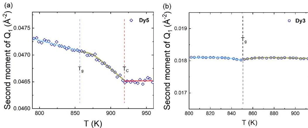
**Fig. S2** Evolution of second moment of  $Q_1$  for (a) Dy5 and (b) Dy3 BMGs. The second moment of  $Q_1$  is correlated with the structural order.
