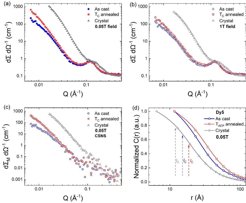
**Fig. S5** One-dimensional plot of total scattering cross section for as-cast,  $T_{\text{AEP}}$ -annealed, and crystal Dy5 at (a) 0.05 T and (b) 1 T field. (c) Corresponding spin-misalignment scattering cross section at 0.05 T. (d) Normalized correlation function for different states of Dy5.
