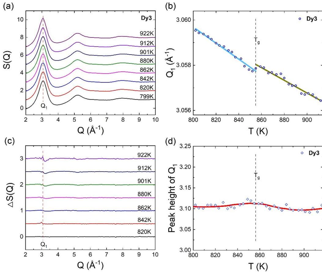
**Figure S1.** (a)  $S(Q)$  for Dy3 MGs. (b) Evolution of peak position  $Q_1$  for Dy3 BMG, showing only one change in slope at  $T_g$ . (c) Evolution of peak height of first diffraction peak for (c) Dy5. (d) Peak height as a function of temperature.
