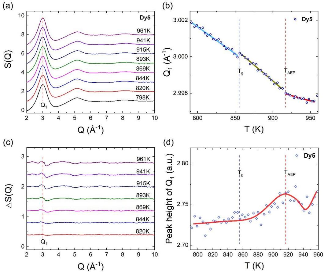
**Fig. 2.** Structure factor of Dy5 bulk metallic glasses: (a)  $S(Q)$  of Dy5 BMG, (c)  $\Delta S(Q)$  in Dy5 BMG, (b) first moment  $Q_1$  and (d) peak height in Dy5 BMG.
