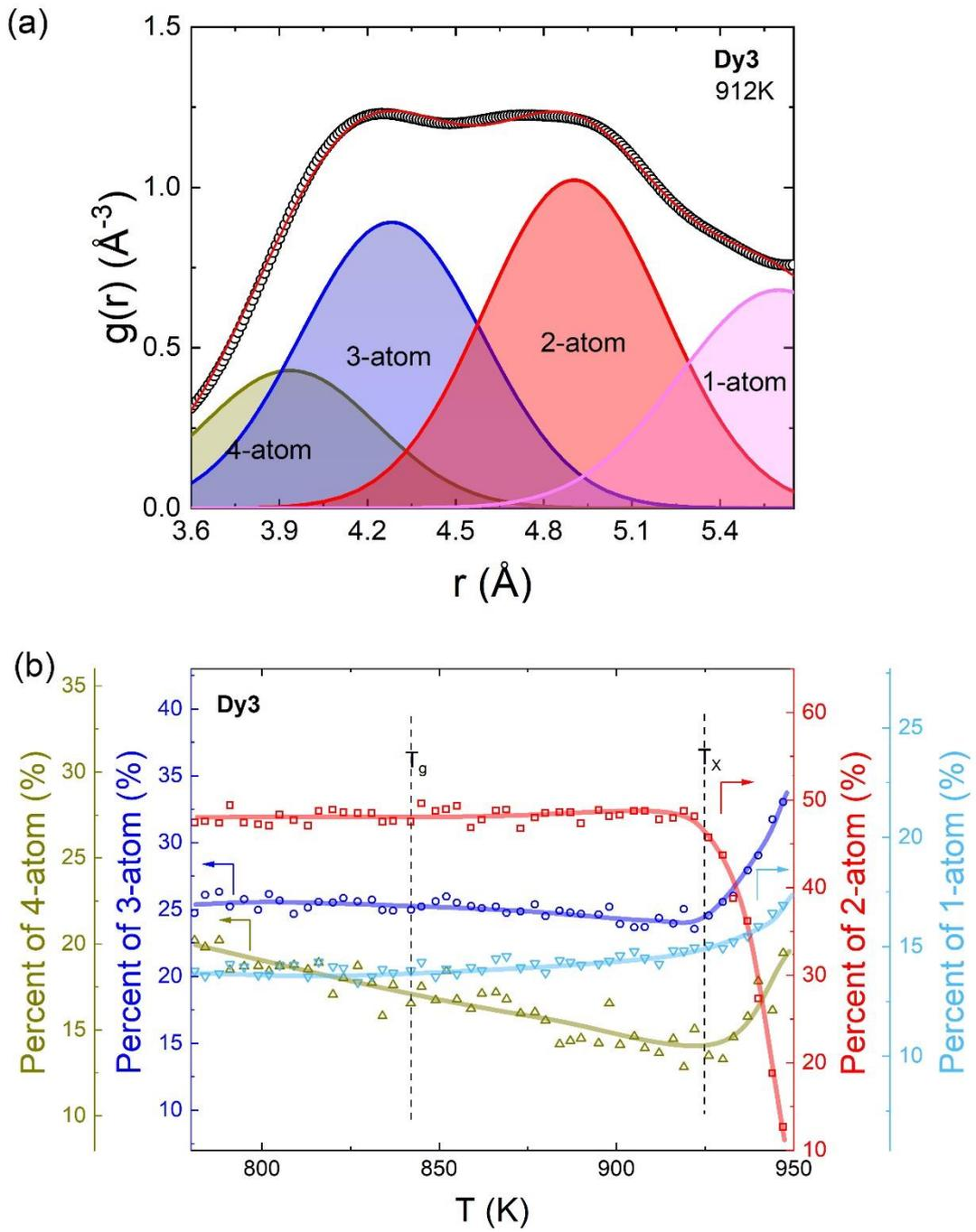
**Fig. S3** (a)  $g(r)$  upon heating Dy<sub>3</sub> BMG and (b) evolution of the corresponding atomic connectivity, showing the percent of connection modes as a function of temperature.
