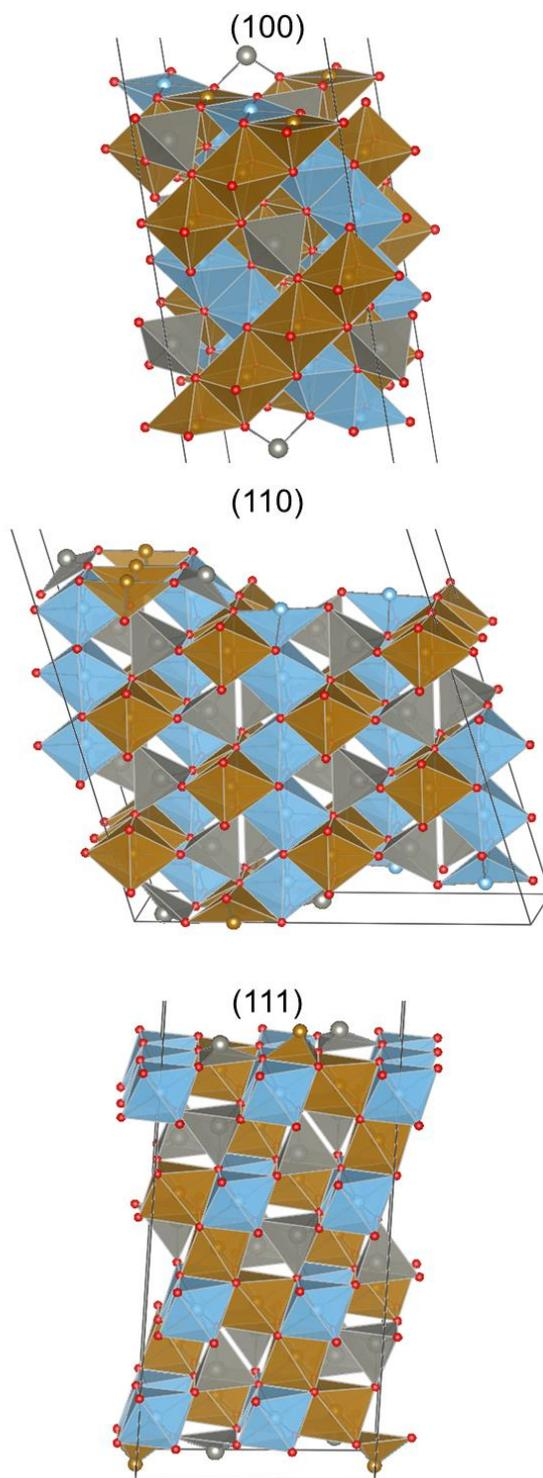
**Fig. 1.** Terminations of  $\text{ZnM}_2\text{O}_4$  surfaces. Gray, brown, blue, and red balls indicate Zn, spin-up M, spin-down M, and O. Spin up and down are not distinguished for  $\text{M}=\text{Al}$ , Ga, In, and Co.
