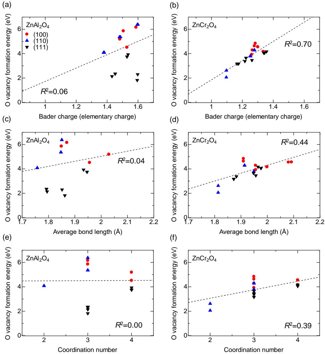
Fig. 4.  $E_{\text{Ovac}}$  versus (a,b) O site Bader charge, (c,d) average bond length, and (e,f) coordination number of desorbing O for (a,c,e)  $\text{ZnAl}_2\text{O}_4$  and (b,d,f)  $\text{ZnCr}_2\text{O}_4$ .
