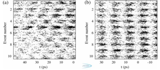
Figure 2: Ten consecutive time-resolved images of the self-modulated  $p^+$  bunch in case of RIF propagating 600 ps (a) and 350 ps (b) ahead of the bunch center. The bunch propagates from left to right.  $n_{pe} = 0.94 \times 10^{14} \text{ cm}^{-3}$ . Figure reproduced from [16].
