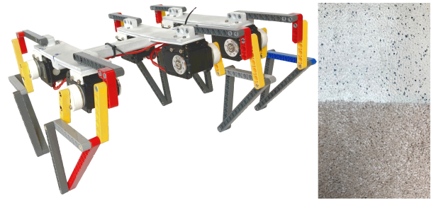
Fig. 2. The hexapod robot platform used for testing the evolved mechanical linkages, and the two floor textures it is tested on.
