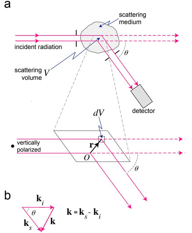
FIG. 7 Schematic of a light-scattering set-up. (a) Global view of the set-up. In the expanded view, scattering through an angle  $\theta$  is indicated in a small volume  $dV$ . (b) Close up of the scattering volume with the scattering wavevector  $\mathbf{k}$  defined in terms of the wavevector of the incident  $\mathbf{k}_i$  and scattered  $\mathbf{k}_s$  light, and also the scattering angle  $\theta$ . Inspired by Pusey (2002).
