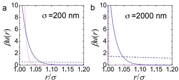
FIG. 5 Estimation of effective colloid-colloid interactions for various hard-sphere-like scenarios for particle diameters (a)  $\sigma = 200$  nm and (b)  $\sigma = 2000$  nm. Shown is steric stabilization (pink line), strong electrostatic interaction (solid blue line) and weak electrostatic interaction (dashed blue line). See text for additional details. Figure reproduced from (Royall *et al.*, 2013).
