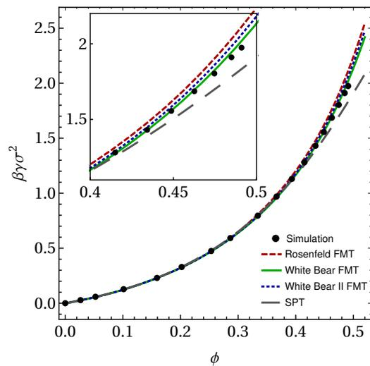
FIG. 18 Interfacial free energy of a hard-sphere fluid in contact with a flat hard wall, as a function  $\phi$ . The lines are theoretical predictions based on fundamental measure theory (FMT) and scaled particle theory (SPT). The points are simulation data. Simulation and FMT data taken from Davidchack *et al.* (2016); the SPT expression is based on Heni and Löwen (1999).
