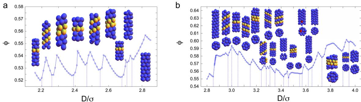
FIG. 27 Close packing fraction of hard spheres confined in cylinders of diameter  $D$  along with some of the structures. These packings (a) are phyllotactic-like for  $D/\sigma \lesssim 2.8$ , and (b) exhibit a core-shell structure beyond that point. Reproduced from (Fu *et al.*, 2016) with permission from the Royal Society of Chemistry.
