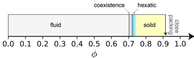
FIG. 16 Hard-sphere phase behavior in 2d as a function of area fraction. Close packing is indicated at  $\phi_{\text{cp}} = 0.907\dots$ . The first-order fluid-hexatic transition is marked by a narrow coexistence region of  $\phi \approx 0.68 - 0.70$ . The hexatic-solid transition is second order at  $\phi \approx 0.73$  as indicated by the shading. Phase boundaries are taken from [Bernard and Krauth \(2011\)](#).
