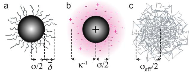
FIG. 4 Schematic representation of various models for hard-sphere colloids. (a) A sterically-stabilized particle has surface “hairs” (not to scale) of average thickness  $\delta$ , resulting in core-stabilizer diameter  $\sigma_{\text{cs}} = \sigma_c + 2\delta$ . (b) A charged colloid has an electrical double layer (shaded) that gives rise to an effective diameter  $\sigma_{\text{eff}}$ . (c) A microgel particle is a heavily cross-linked polymer. Figure reproduced from (Royall *et al.*, 2013).
