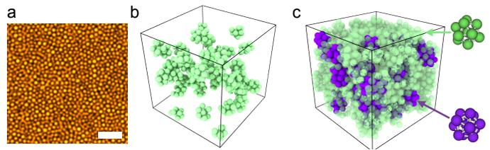
FIG. 37 Resolving small colloids in real space. **a**, STED nanoscopy image for  $\phi = 0.598$ . Scale bar corresponds to  $3 \mu\text{m}$ . **b,c**, Rendered coordinates of defective icosahedra (green, top right structure) and full icosahedra (purple, bottom right structure) for **(b)**  $\phi = 0.523$  and **(c)**  $0.598$ , respectively. Reprinted from Hallett *et al.* (2018) under Creative Commons Attribution 4.0 International License <http://creativecommons.org/licenses/by/4.0/>.
