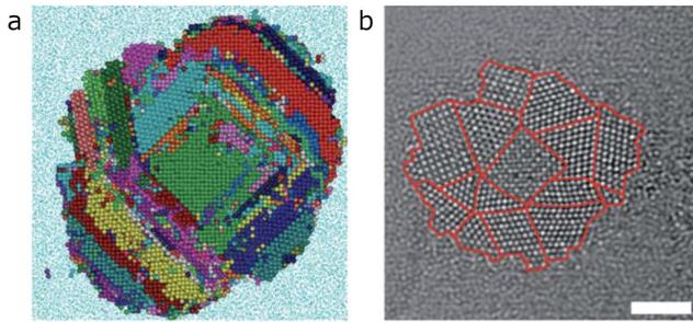
FIG. 48 Seeding a hard-sphere crystal from a square seed in (a) simulations at  $\phi = 0.51$ , and (b) experiments with optical tweezers. In (a), the colors correspond to different crystal grains, crystalline particles are drawn at their normal size, while fluid particles are drawn as dots. In (b), the scale bar is  $10 \mu\text{m}$ . Reproduced from (Hermes *et al.*, 2011) with permission from the Royal Society of Chemistry.
