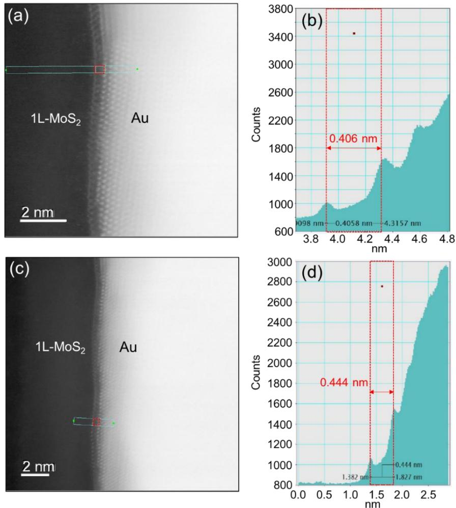
**Figure 4:** (a,c) Aberration corrected STEEM/HAADF analyses of 1L-MoS<sub>2</sub>/Au interface. (b,d) Intensity line profiles, from which the atomic distance between the Mo atoms of the MoS<sub>2</sub> membrane and the topmost Au atoms was evaluated.
