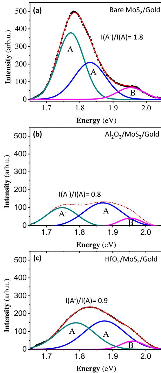
**Figure 11:** Micro-PL spectra on the bare 1L-MoS<sub>2</sub>/Au (a) and after 80 ALD cycles of Al<sub>2</sub>O<sub>3</sub> (b) and HfO<sub>2</sub> (c). The deconvolution of the PL peak results in three different contributions: the trion peak  $A^-$ , the exciton A, the exciton B.
