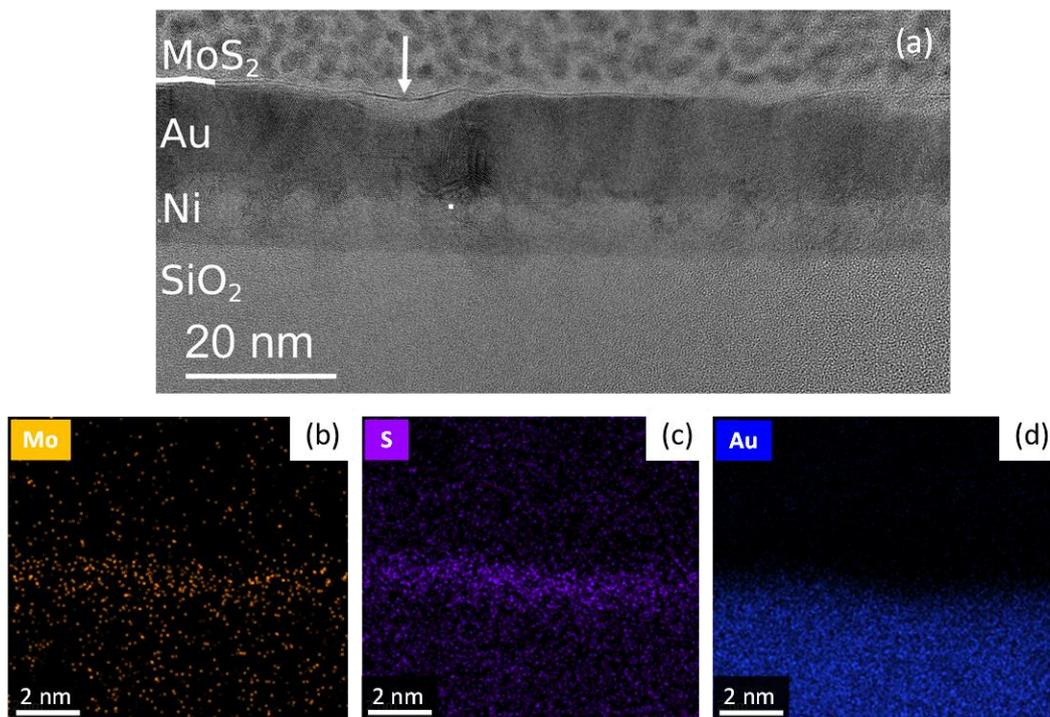
**Figure 3:** (a) Low magnification TEM analysis of the monolayer MoS<sub>2</sub> membrane on the Au/Ni/SiO<sub>2</sub> stack. EDS maps of Mo (b), S (c), Au (d) acquired on the magnified MoS<sub>2</sub>/Au region.
