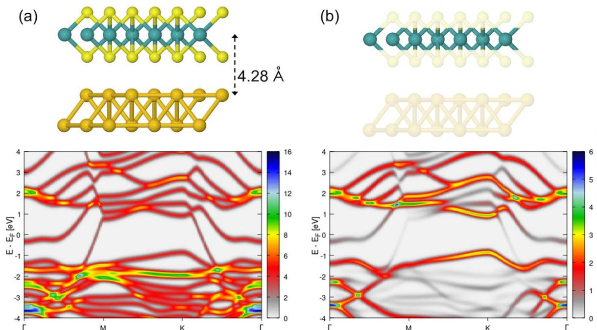
**Figure 5:** Structure and electronic properties of the MoS<sub>2</sub>/Au(111) interface showing the (a) the total k-resolved projected density of states, and (b) the partial k-resolved projected density of states only for Mo 4d orbitals.
