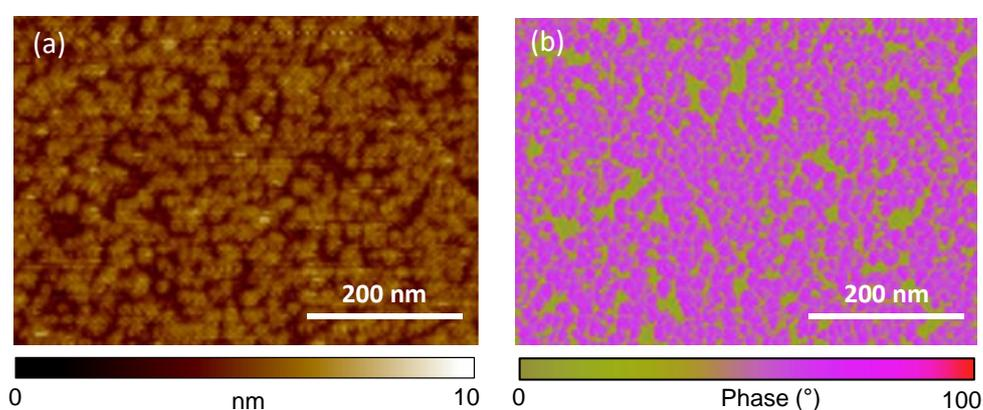
**Figure 6:** Comparison of AFM morphology (a) and phase (b) of 40 ALD cycles HfO<sub>2</sub> on MoS<sub>2</sub>/Au
