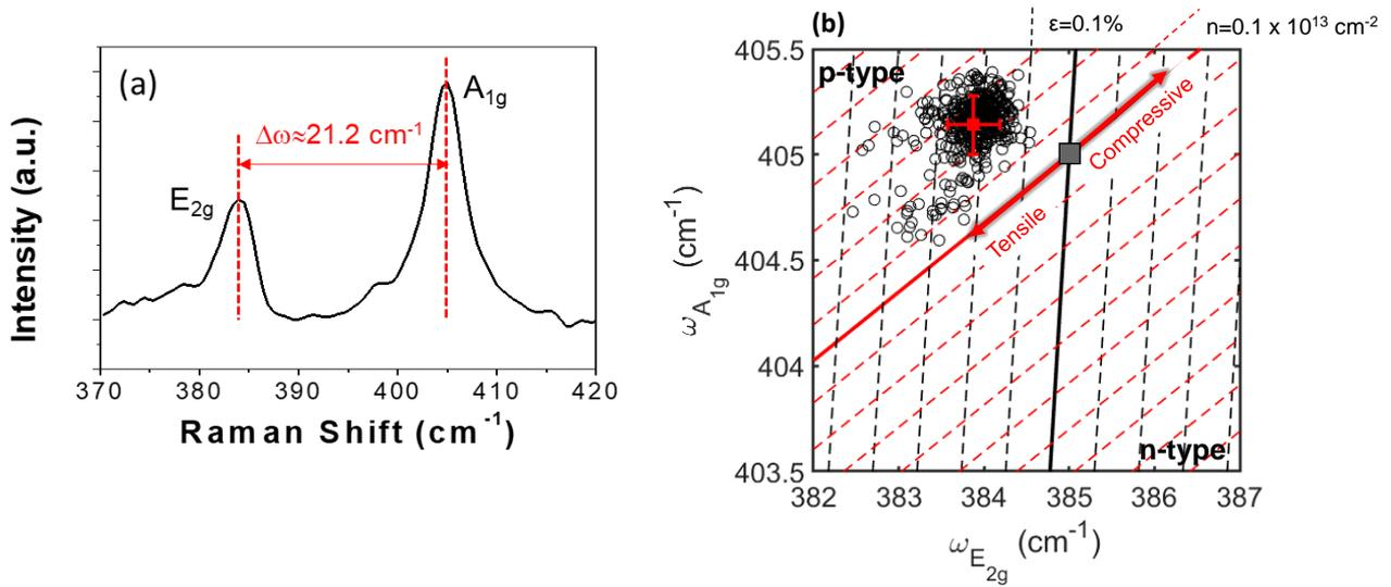
**Figure 2** (a) Typical Raman spectrum of 1L-MoS<sub>2</sub> exfoliated on Au, with the indication of the characteristic in-plane (E<sub>2g</sub>) and out-of-plane (A<sub>1g</sub>) vibrational modes and their separation  $\Delta\omega \approx 21.2$  cm<sup>-1</sup>. (b) Correlative plot of the  $\omega_{A_{1g}}$  and  $\omega_{E_{2g}}$  peak frequencies extracted from an array of Raman spectra measured at different positions on the 1L-MoS<sub>2</sub>/Au sample.
