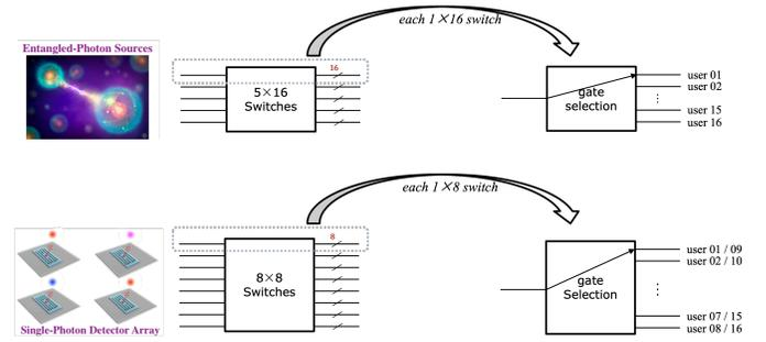
(b) Configuration of the quantum routers for photon routing control.
