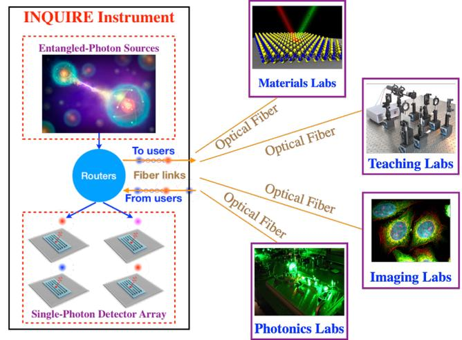
Fig. 1. The deployed INQUIRE instrumental system serves versatile research and teaching objectives via fiber-based transmission of quantum signals. INQUIRE consists of high-quality EPS and SPD resources and quantum routers controlling photon streams between terminal labs and the hub.
