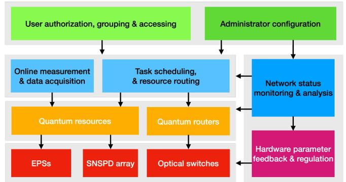
Fig. 6. Architecture and functional modules of Quagent. From bottom to up, they are the hardware layer, resource layer, scheduling layer and user administration layer. Additional modules (right part of the figure) aim at regulating and monitoring the whole platform.
