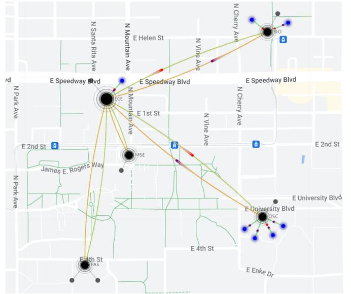
Fig. 4. Real-time dynamic status of network testbed. Quagent is serving multiple users (lab nodes) simultaneously. Rippling blue nodes represent active users occupying EPS or SPD channel resources; grey nodes represent inactive users; large rippling black circles are hubs located in five buildings while ECE is the central hub. Tailing red circles represent entangled-photon streams; tailing purple circles represent single photons from users to be detected.
