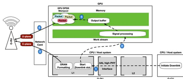
Figure 6 Illustration of downlink data and control flows
