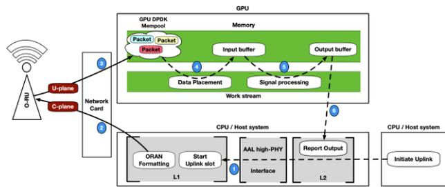
Figure 5 Illustration of uplink data and control flows
