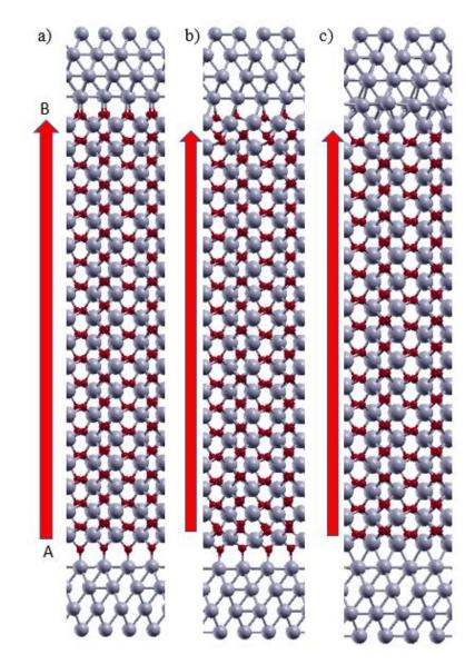
**Figure S4** Atomic configuration of single domain structures with a) vacancy-free O-ended interfaces b) interfaces with one spacer and one polar vacancy c) Hf/Zr-ended interfaces. A and B interfaces are marked as bottom and top interfaces respectively.
