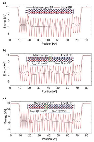
**Figure 7** Plane averaged local and macroscopic electrostatic potential along the polarization direction for 4.58 nm thick HZO in MFM when a) HZO is in SD state b) DW is at the center c) DW is one unit cell away from the center. Insets show the corresponding atomic configurations. At SD state there is negligible depolarization field as opposed to finite values in MD state. Depolarization field increases in the narrower domain when DW shifts from the center.
