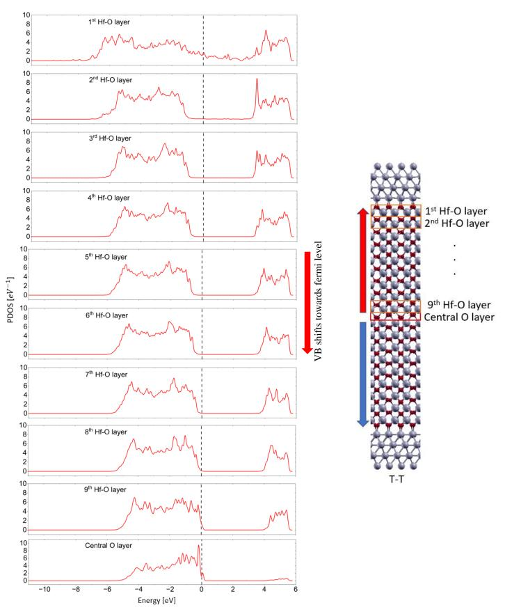
**Figure S3** Layer wise PDOS from the interfacial Hf-O atoms towards the central O atoms at the DW for T-T configuration. VB shifts towards the fermi level as we move towards the DW region which indicates that holes appear near the DW. (The first Hf-O layer is interfacial; therefore, they are metalized and corresponding projected bandgap is not observable.)
