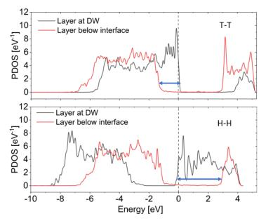
**Figure 6** PDOS of atomic layers below the interface and at the DW of unrelaxed a) T-T and b) H-H configurations with relaxed vacancy-free O-ended interface. The arrows represent the bend bending needed to accumulate necessary free carriers for bound charge compensation at the DW. Thus, higher depolarization field is needed for stabilizing H-H DW.
