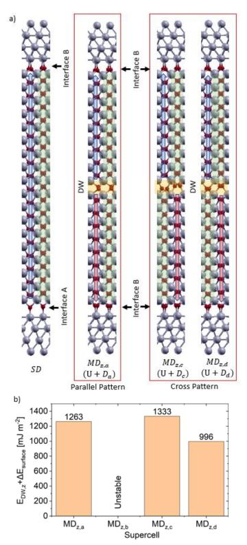
**Figure 2** Atomic configurations of MFM HZO samples for O-ended interface without vacancy a) Single domain and multidomain T-T supercells consisting of U and  $D_a$ ,  $D_c$  and  $D_d$  of Figure 1 respectively. Combination of U and  $D_b$  is unstable. b) Total energy difference with SD for each MD structure. The energy values in the bar include the difference between SD and MD interface energy as well as the DW energy. Thus, cross-pattern  $MD_{z,d}$  gives the lowest energy.
