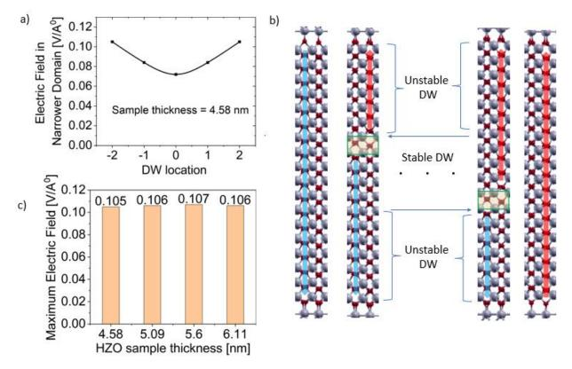
**Figure 8** a) Depolarization field in the narrower domain with the position of the DW away from the center in terms of half-unit cell. b) Regime of stability of DW. DW is only stable within a certain distance from the center. Beyond that point, the excess depolarization filed destabilizes the DWs. c) Consistency of the magnitude of maximum depolarization field with varying HZO sample thickness.
