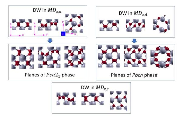
**Figure S2** Atomic configuration of DWs in Figure 2. All the DWs are half unit cell thick and so half-cell thick configuration is shown here. The DWs in  $MD_{z,a}$  and  $MD_{z,c}$  are orthorhombic  $Pca2_1$  phase and 90° rotated with respect to the domains. The DW in  $MD_{z,d}$  resemble orthorhombic *pbcn* phase. For better comparison purpose, planes of full unit cell of  $Pca2_1$  and *pbcn* phases are also demonstrated.
