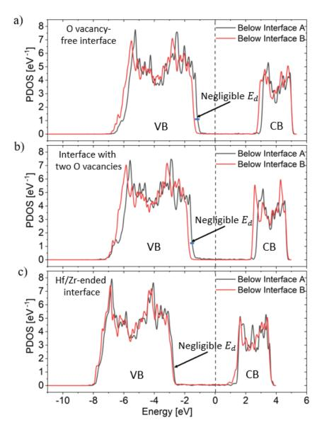
**Figure S5** Projected Density of States (PDOS) of atomic layers of SD HZO adjacent to the two interfaces for a) O-ended interfaces without vacancy b) interfaces with one spacer and one polar vacancy c) Hf/Zr-ended interfaces shown in Figure S4a-c respectively. The negligible shift between the bands near the two interfaces dictates negligible depolarization field, i.e., excellent bound charge screening by metal irrespective of oxygen vacancy density.
