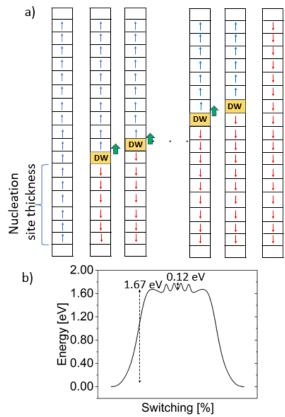
**Figure 10** a) Schematics of nucleation and DW motion for polarization reversal through T-T DW. Arrow in each slot represents polarization of half-unit cell along the polarization direction. The empty slot represents interface oxygen layer. Minimum nucleation site thickness is 1.63 nm (3 unit cell thick). b) Barrier height for polarization reversal. Nucleation barrier per unit cell is 1.67/3 = 0.55 eV and DW motion barrier per unit cell is  $0.12 \times 2 = 0.24$  eV.
