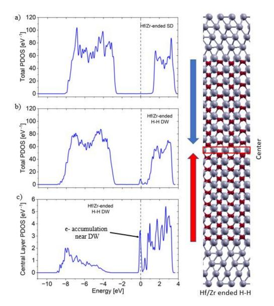
**Figure S7** Total PDOS of atomic layers of a) SD HZO and b) MD HZO of H-H configuration for Hf/Zr-ended interfaces c) PDOS at central Hf/Zr layer for H-H DW configuration in HZO. The CB minimum and fermi level suggest that electrons appear at the DW to screen positive polarization bound charges. This comes at the cost of depolarization field inside the domains. The structure at the right side shows the abovementioned H-H structure.
