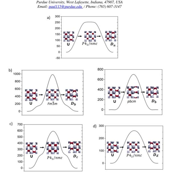
**Figure S1** a)-d) Polarization reversal path for upward polarized unit cell, U to downward polarized unit cells  $D_a$ ,  $D_b$ ,  $D_c$  and  $D_d$  respectively. The unit cells are taken from Figure 1 of main text. From U to  $D_b$  transition, both  $Fm\overline{3}m$  and pbcm can occur as intermediate state as shown in the two paths of b). For U to  $D_a$ ,  $D_c$  and  $D_d$  transition,  $P4_2/nmc$  occurs as the intermediate phase.
