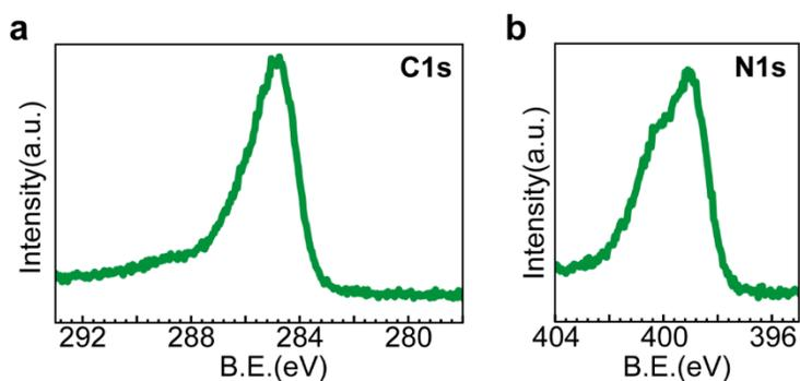
**Figure 3.** XPS spectrum of (a) C1s and (b) N1s from the powder sample on copper substrate. Each spectrum was normalized at each peak top.
