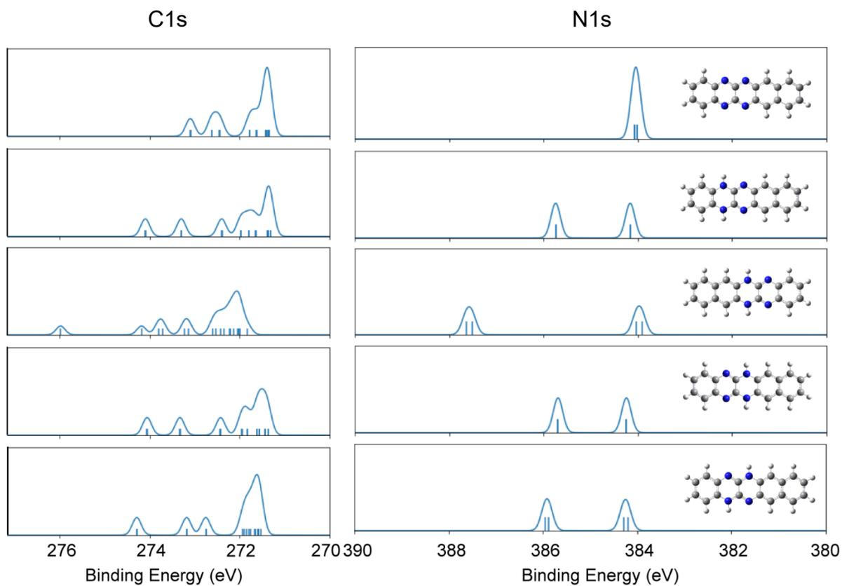
**Figure S1.** Quantum chemical calculation results of C1s and N1s of a single BTANC and H<sub>2</sub>BTANC molecules.
