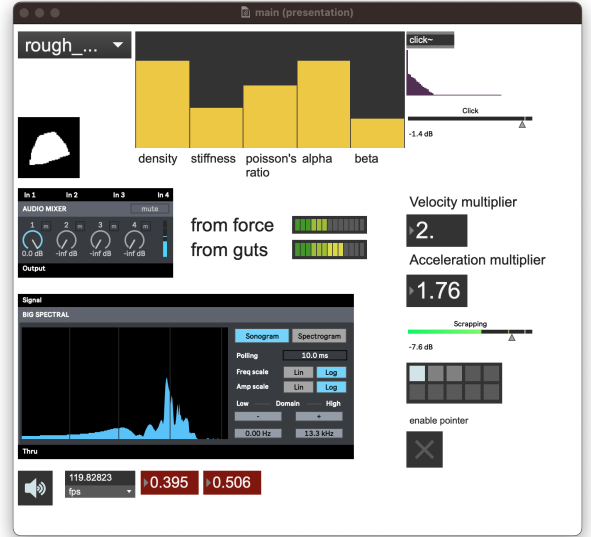
Figure 1: Prototypical user interface in Max/MSP. On the left, the interface for shape deformation is displayed. The user is able to deform a 2D mesh by moving vertex handles or generating a random mesh. They can also interact with the resonator by sliding or scraping inside the shape with the mouse or by clicking an arbitrary point (hitting). On the right, the interface for controlling excitation and material parameters is shown.
