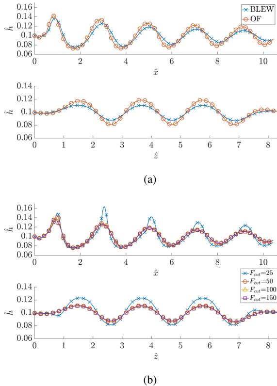
FIG. 9: Comparison in terms thickness profiles along  $x$  (top) and  $z$  (bottom) predicted by IBL and DNS (a), and sensitivity of the results to the cut-off parameter  $F_{cut}$  of the Butterworth filter (b). The test case is the one in Fig. 8 but with larger perturbation ( $A = 0.2$ ) and including the surface tension.
