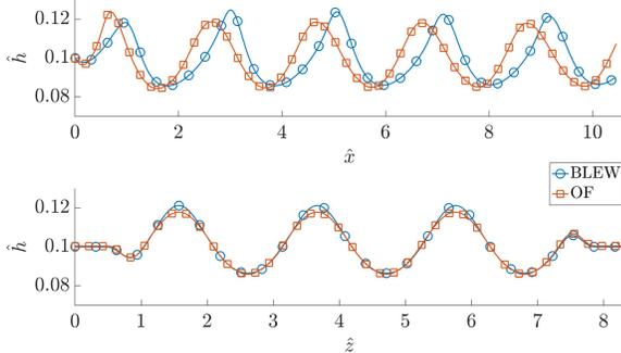
FIG. 8: Comparison between the IBL simulations (in BLEW) and the DNS simulations (in OpenFOAM, OF) in the absence of surface tension. The stream-wise ( $x$ ) thickness evolution is displayed on the top, and the span-wise ( $z$ ) on the bottom.
