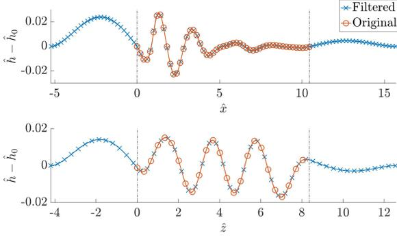
FIG. 2: Original thickness profiles along the stream-wise  $\hat{x}$  (top) and span-wise  $\hat{z}$  (bottom) coordinates together with the smoothed version  $\mathcal{F}^{-1}(HH_F)$  used to compute the capillary terms. Outside the black dashed lines, the original thickness profiles are extrapolated and periodicity is enforced at both sides. The data correspond to the validation test case with surface tension in Section IV B.
