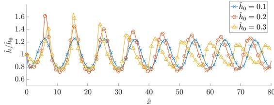
FIG. 13: Stream-wise evolution of three liquid films characterized by  $\delta = 153$  and with a dimensionless frequency of  $\hat{f} = 0.1$  and amplitude of  $A = 0.2$  as in Ivanova et al.<sup>38</sup>, except for  $\hat{h}_0 = 0.3$  in which the amplitude has been fixed at 0.1 to avoid breakup of the wave crest. The vertical axis has been normalized with the nominal film thickness  $\hat{h}/\hat{h}_0$ .
