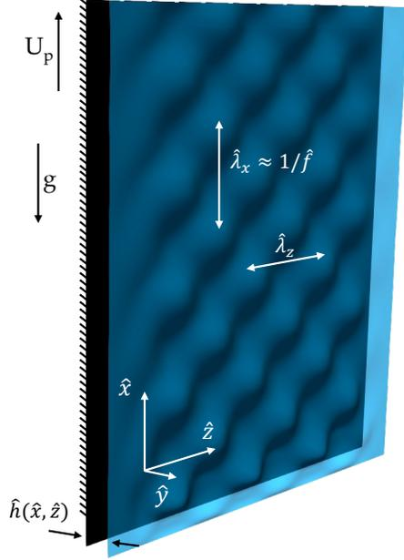
FIG. 1: Schematic of the flow configuration investigated in this work with relevant quantities. The reference frame is chosen so that the stream-wise direction  $\hat{x}$  is aligned with the substrate (upward) velocity,  $U_p$ , and opposite to the gravitational acceleration,  $g$ , although the IBL model is derived considering  $x$  in the direction of gravity for consistency with the literature of falling film models.
