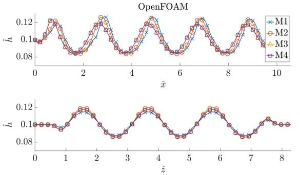
(a) M1 (1.2 M cells):  $n_\lambda = 50$ ,  $n_h = 11$ ; M2 (8.8 M cells):  $n_\lambda = 100$ ,  $n_h = 22$ ; M3 (22.4 M cells):  $n_\lambda = 125$ ,  $n_h = 40$ ; M4 (35.3 M cells):  $n_\lambda = 150$ ,  $n_h = 45$ .
