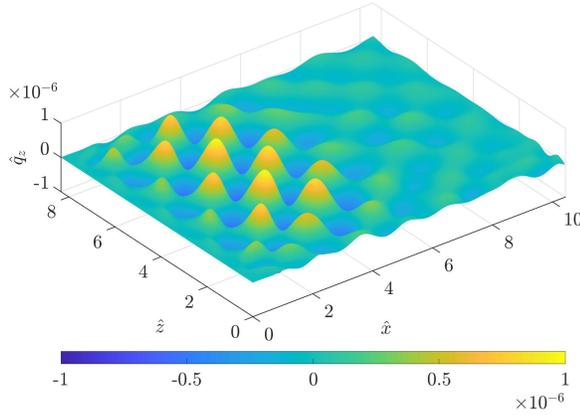
FIG. 12: Spatial evolution of the span-wise flow rate  $\hat{q}_z$  for the base case ( $\hat{k}_x = 3, \hat{k}_z = 3$ ) when surface tension is activated in the IBL solver. The same computation in absence of surface tension leads to  $\hat{q}_z = 0$  everywhere, and therefore it is not included here.
