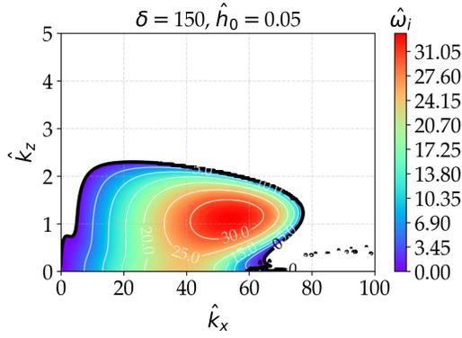
FIG. 5: Same plot as in Fig. 4, for the case with  $\delta=150$  and  $\hat{h}_0=0.05$ . The white area is the stable region ( $\hat{\omega}_i < 0$ ). Above  $\hat{k}_x > 80$  and  $\hat{k}_z > 2.5$ , all waves are linearly stable because of surface tension.
