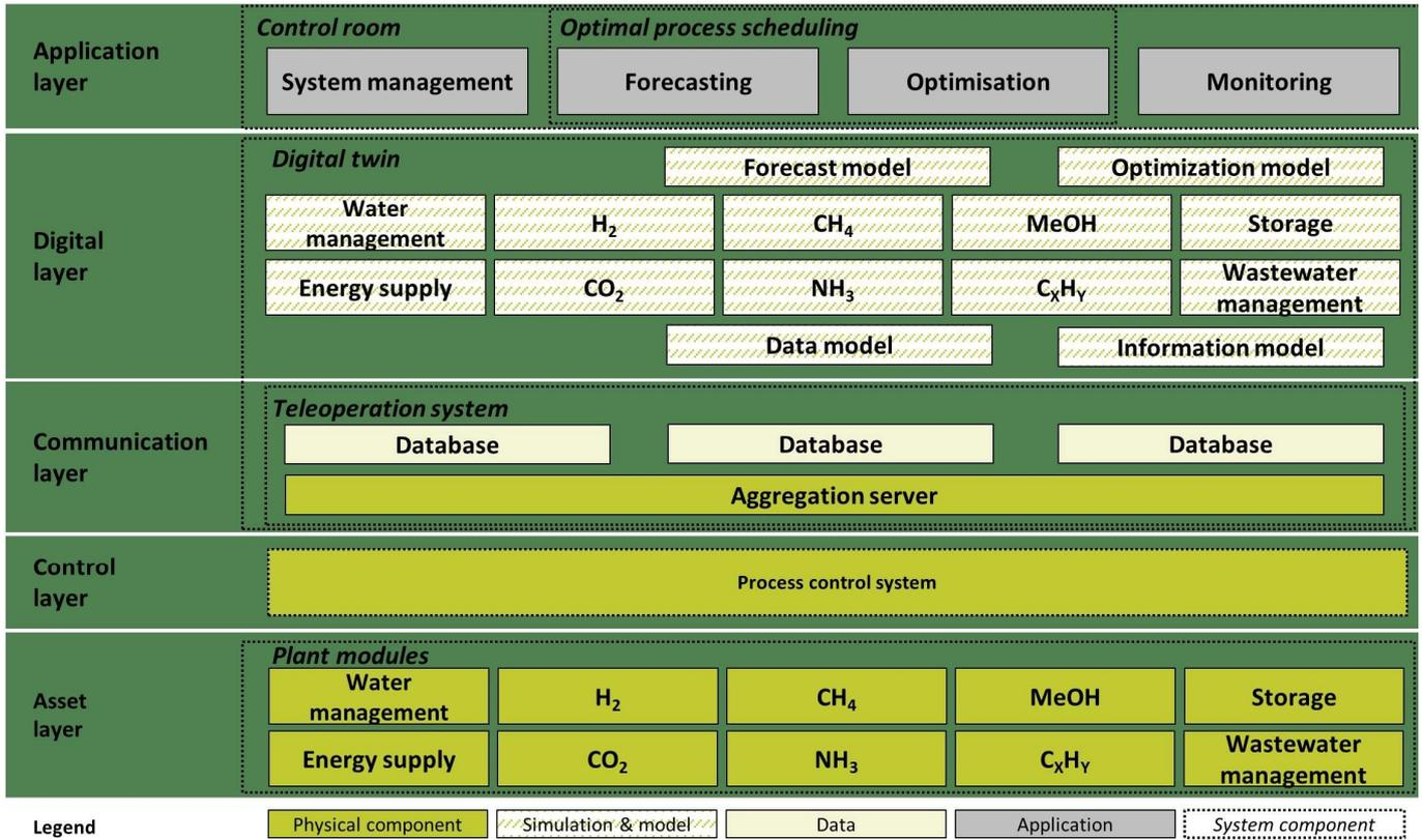
Figure 1. System architecture for a modular production platform with five layers based on [15].
