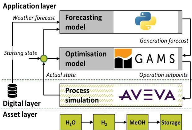
**Figure 3.** Simplified prototype for an optimal process scheduling using the example of a power-to-methanol process.
