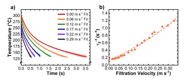
**Supporting Figure 7**: a) Selection of cooling curves with corresponding fits for various fluid velocities b) Inverse of  $\tau_2$  of Equation (8) with quadratic fit
