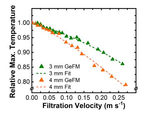
Supporting Figure 8: Maximum temperature during heat pulse over fluid velocity with quadratic fit
