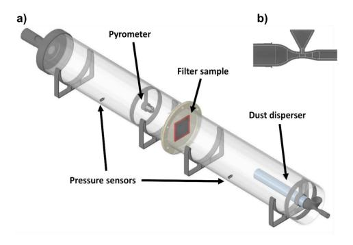
**Supporting Figure 9: a)** Wind-tunnel setup for load detection measurements including self-designed dust dispenser as well as sensing periphery. **b)** Cross-section of the dust dispensing venturi nozzle
