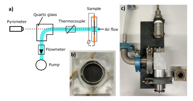
Supporting Figure 6: Flowmeter capability measurement setup a) Scematic of the setup b) filter material sample in holder c) Photograph of the setup
