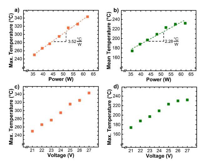
Supporting Figure 4: Joule-Heating characteristics of filter material **a-b**) Maximum and mean temperature versus applied power including linear fits **c-d**) Maximum and mean temperature versus applied voltage.
