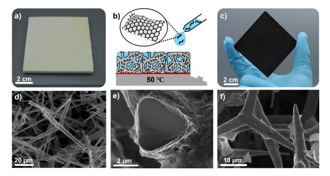
**Figure 2: a)** Photograph of 68x68x4 mm ZnO network for preparation of the filter medium **b)** Schematic of the drop infiltration process **c)** Photograph of finished graphene-enhanced filter medium. Cross-sectional SEM images: **d)** Pristine ZnO network **e)** Tetrapod arm after the infiltration process, showing the deposited graphene thin film **f)** Network of graphene-enhanced filter medium.
