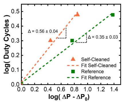
**Supporting Figure 5:** Double logarithmic plot of use duty cycles versus pressure drop increase. Linear fits are applied to extract the gradient for further calculations.
