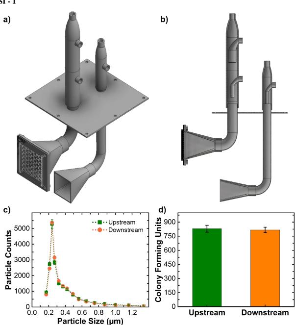
**Supporting Figure 1:** Nozzle setup for filter measurements **a**) Isometric view **b**) Cross-sectional view. Positive measurements of **c**) particle spectra for the nozzle system. **d**) Bacillus subtilis
