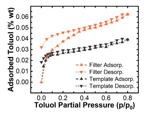
**Supporting Figure 3**: Gravimetric adsorption of Toluene measured with nitrogen carrier gas at an overall gas flow of 100 sccm/min
