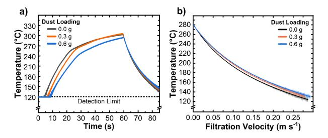
**Supporting Figure 10: a)** Complete temperature response curves of GeFM samples when loaded with three different amounts of test dust. **b)** Cooling curves with bi-exponential fit for GeFM loaded with three different amounts of test dust.
