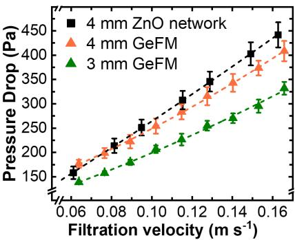
**Supporting Figure 2:** Pressure drop curves of GeFM of different thickness compared to the pristine base ZnO base network with quadratic fit
