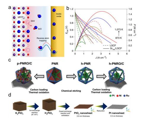
**Figure 22.** Topotactic transition for application of fuel cells. a) Schematic of SrO captured by acidic MoO<sub>3</sub> to transform topotactically to SrMoO<sub>4</sub>. b) The performance of SOFCs with LSFC and strontium-deficient LSCF. Reproduced with permission.<sup>[143]</sup> Copyright 2022, Springer Nature. c) Schematic illustration of the topotactic transition for fabricating Pt/RuO<sub>2</sub>
