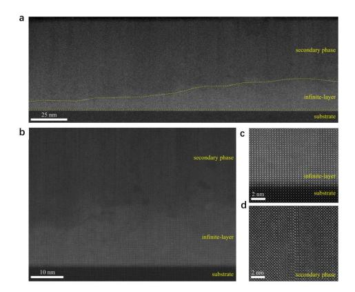
**Figure 18.** HAADF-STEM image of the obtained NSNO thin film. a) image of the mixedphase film with substrate after the reduction. b) Magnified image of panel (a) with two phases. c) Magnified image of panel (b) in the infinite-layer region. d) Magnified image of panel (b) in the secondary phase region. Reproduced with permission.<sup>[113]</sup> Copyright 2020, American Institute of Physics.
