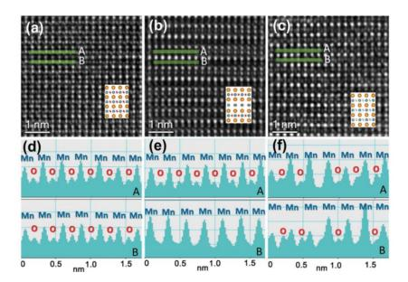
**Figure 9.** Structural characterization of different LSMO phases. HRTEM image of a) PV-LSMO b) BM-LSMO and c) oxygen deficient PV-like LSMO structure phases. The insets show corresponding structural models for each image (La/Sr: yellow, Mn: green, O: red in a) and b), grey in c)). d)-f) Line profiles of two neighboring Mn-O layers indicated by green AB line in the HRTEM images. Reproduced with permission.<sup>[65]</sup> Copyright 2014, Wiley-VCH.
