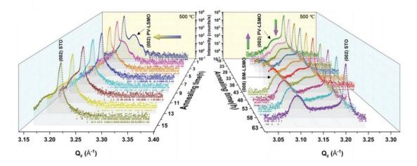
**Figure 8.** *In-situ* XRD scans of the 45-nm-thick  $La_{0.7}Sr_{0.3}MnO_{3-\delta}$  film on a STO substrate in 500 °C with increasing annealing time. Reproduced with permission.<sup>[62]</sup> Copyright 2019, Wiley-VCH.
