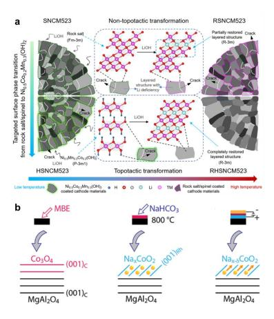
**Figure 23.** The application of the topotactic transition in ion batteries. a) Mechanisms for the regeneration of  $LiNi_{0.5}Co_{0.2}Mn_{0.3}O_2$  via topotactic transition. Reproduced with permission.<sup>[150]</sup> Copyright 2023, American Chemical Society. b) Schematic of the synthesis process of  $Na_xCoO_2$  through the topotactic transition. Reproduced with permission.<sup>[153]</sup> Copyright 2023, American Chemical Society.
