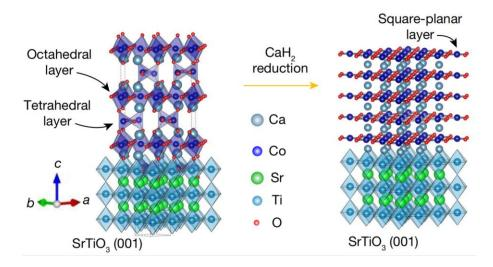
**Figure 16.** Crystal structure of precursor BM CaCoO<sub>2.5</sub> (left) and product CaCoO<sub>2</sub> (right) on (001) oriented STO substrate by the topotactic CaH<sub>2</sub> reduction. Reproduced with permission.<sup>[98]</sup> Copyright 2023, Springer Nature.
