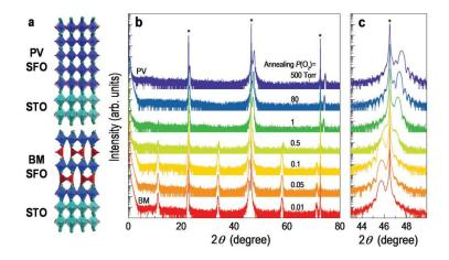
**Figure 12.** Crystal structure of SrFeO<sub>x</sub> (SFO) epitaxial thin films. a) Crystal structure of PV-SFO and BM-SrFeO<sub>2.5</sub> thin films on STO substrate. b) and c) XRD patterns of SFO thin films with different annealing oxygen pressure. Reproduced with permission.<sup>[70]</sup> Copyright 2017, Wiley-VCH.
