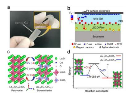
**Figure 15.** The description of IG gating-modulation process. a) Photos of the bending of IG. b) Schematic diagram of all-solid-state IG gating-modulation process. c) Reversible topotactic transition between PV-LSCO and BM-LSCO. d) Energy gap between PV-LSCO and BM-LSCO calculated by theoretical calculations. Reproduced with permission.<sup>[95]</sup> Copyright 2022, American Physical Society.
