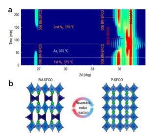
**Figure 14.** Topotactic transition in SFCO system. a) Gas-type-dependent real-time XRD  $\theta$ -2 $\theta$  measurement at 375 °C. b) Schematic diagram of reversible redox reaction in SFCO. Reproduced with permission.<sup>[78]</sup> Copyright 2018, American Physical Society.
