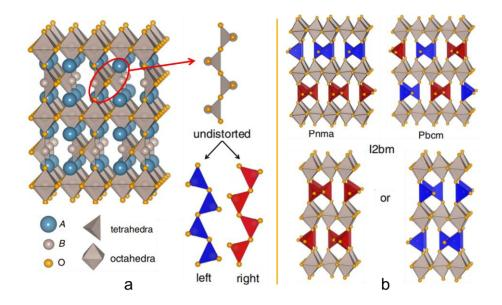
**Figure 1.** The structure of a BM phase with different space groups. a) The crystal structure of the BM phase and the two types of tetrahedra chains marked by red and blue. b) The structure of the BM phase belongs to Pnma, Pbcm and I2bm space groups, respectively. Reproduced with permission.<sup>[24]</sup> Copyright 2015, American Physical Society.
