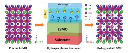
**Figure 10.** Schematics of pristine PV-LSMO films experiencing electrical injection of protons to transform into BM-LSMO. Reproduced with permission.<sup>[66]</sup> Copyright 2019, Wiley-VCH.
