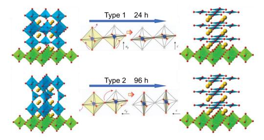
**Figure 2.** The two types of oxygen migration patterns of the topotactic transition from SrFeO<sub>2.5</sub> to infinite-layer SrFeO<sub>2</sub>. Reproduced with permission.<sup>[39]</sup> Copyright 2012, Chemical Society Reviews.
