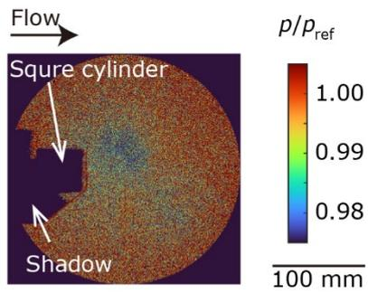
**Figure 2.** Typical pressure distribution, where pressure  $p$  is normalized by an atmospheric pressure  $p_{\text{ref}}$ . Reproduced from Inoue et al.<sup>31</sup>.
