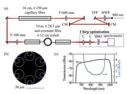
Fig. 1. (a) Sketch of the experimental setup. HWP: half-wave plate, TFP: thin-film polarizer, CM: chirped mirror,  $f_1$ : 100 mm collimating lens,  $f_2$ : 150 mm focusing lens. (b) fiber cross section with 28.3 µm core diameter. (c) fiber transmission (black) as measured for 10 m fiber length, and attenuation (blue) [12].
