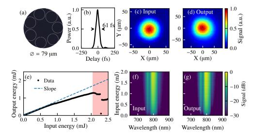
Fig. 8. (a) Cross-section of the larger-core (79 µm diameter) anti-resonant fiber used to scale the input energy. (b) Input pulse and input (c) and output (d) near-field beam profiles. (e) Energy transmission of large-core fiber, with slope efficiency (dashed blue) of 85%. The shaded area annotates the energy regime where guidance is lost. Input (f) and output (g) spectra with increasing energy.
