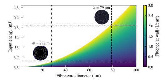
Fig. 7. Below-threshold fluence (up to  $3 \, \text{J/cm}^2$  for 40 fs long pulses) at the fiber core-wall with respect to input energy and fiber core diameter, as calculated using Eq. 1. The dotted lines annotate the maximum energy predicted for a 28  $\mu$ m diameter fiber and the dashed lines annotate the maximum energy predicted for a 79  $\mu$ m diameter fiber.
