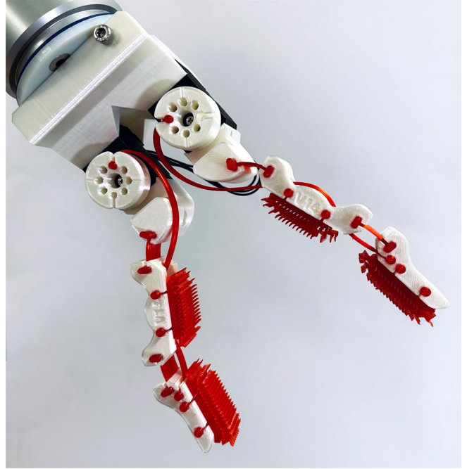
Figure 1: The underactuated InstaGrasp features rigid and flexible components that are 3D printable on hobby grade machines. The only screws used are packaged with the actuators. All parts apart from actuators and those screws are 3D printed.
