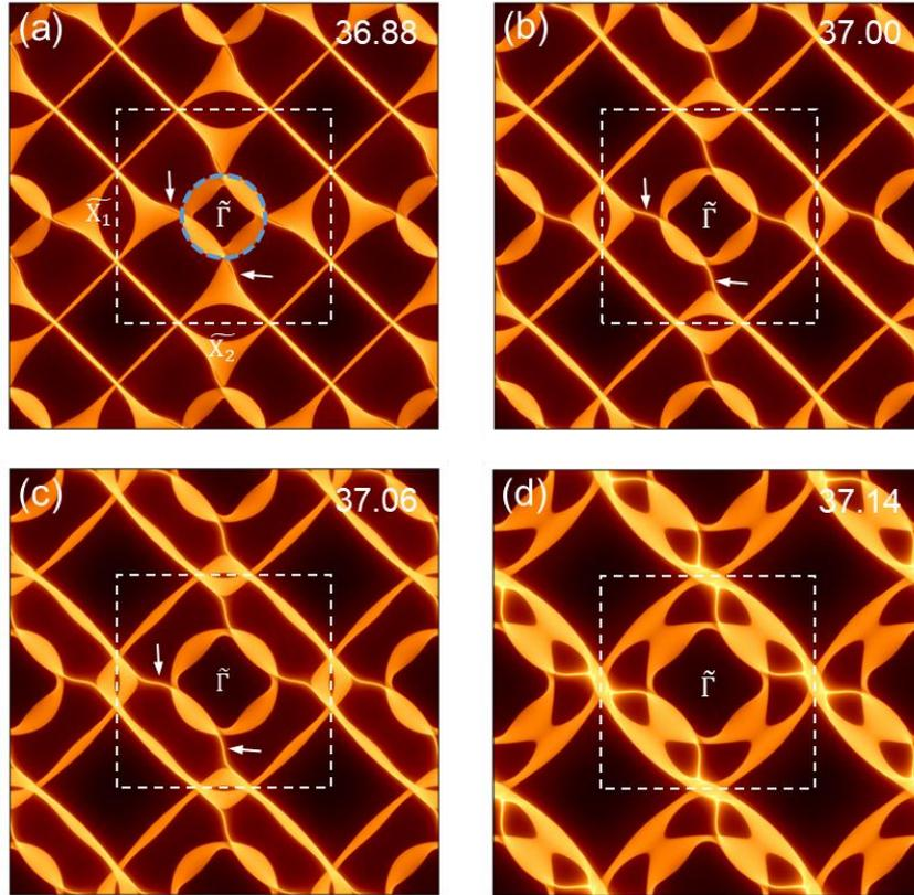
**Figure S6.** Ribbon-like SSs from one NS to another. (a) The SSs begin to emerge at 36.88 THz upon the central intermediate bulk states (light blue circle) are gapped away from the projections of two NSs. The iso-frequency (001) surface contours at (b) 37.00 THz; (c) 37.06 THz and (d) 37.14 THz. In (d), The SSs begin to disappear when the projections of two NSs and central intermediate bulk states are connected.
