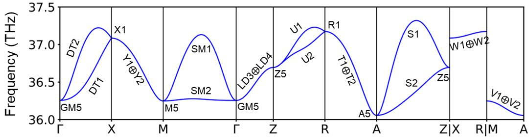
**Figure S4.** Irreducible representations of phonon bands 27,28 of C<sub>4</sub>N, where the convention follows Bilbao crystallographic server <https://www.cryst.ehu.es/>.
