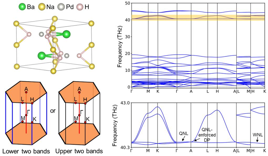
**Figure S41.** The 1NS+QNL+WNL and 1NS+QNL phonons in mp-862693  $\text{BaNaH}_3\text{Pd}$  (SG 194), without LOTO.
