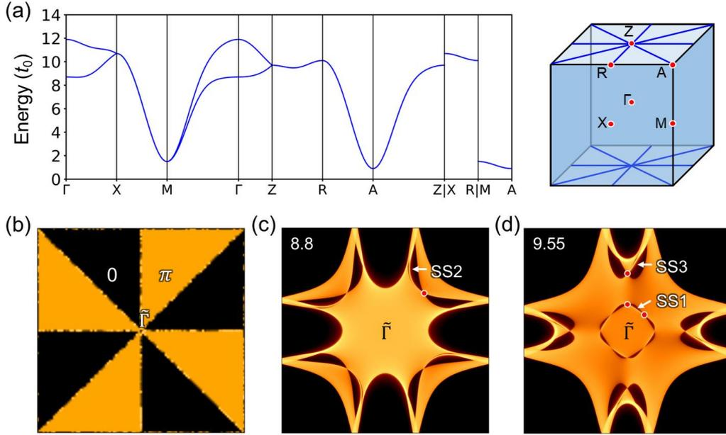
**Figure S2.** TB model of SG 128. (a) Phonon dispersions with  $\Delta = 8.0$ ,  $t_1 = 1.0$ ,  $t_2 = -0.6$ ,  $t_3 = -0.2$ ,  $t_4 = 0.15$ ,  $t_5 = 0.1$  and  $t_6 = 0.0$ , in unit of  $t_0$ . (b) Zak phase  $Z(k_x, k_y)$  of band 1. The right inset shows the 2NS+WNN phonon. The iso-frequency contours of (001) surface at (c)  $E = 8.8t_0$  and (d)  $E = 9.55t_0$ .
