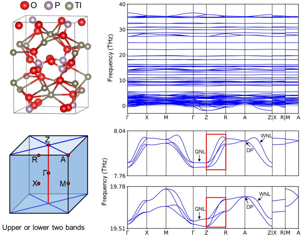
**Figure S42.** The 2NS+HNN phonons in mp-27144 TIPO<sub>3</sub> (SG 114), without LOTO. The red boxes mark the hourglass phonons. The DPs are caused by an irreducible representation of  $A_5^2 \oplus A_5^2$ .
