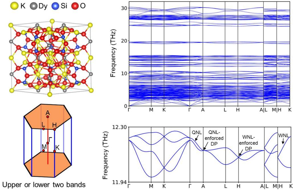
**Figure S40.** The 1NS+QNL+WNL phonons in mp-16595  $\text{K}_3\text{DySi}_2\text{O}_7$  (SG 193), without LOTO.
