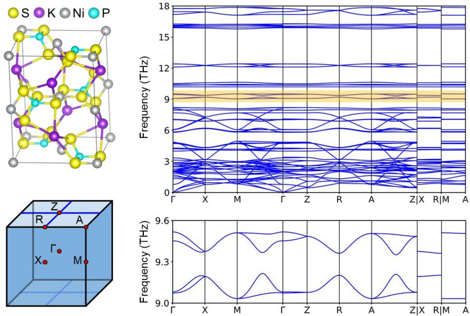
**Figure S21.** The 2NS+WNN phonons of mp-662530  $\text{KNiPS}_4$  (SG 136), with LOTO.
