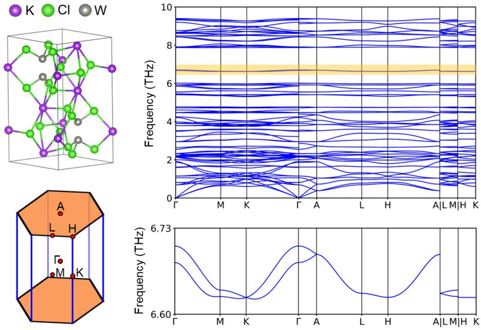
**Figure S23.** The 1NS+WNL phonon of mp-27506  $\text{K}_3\text{W}_2\text{Cl}_9$  (SG 176), with LOTO.
