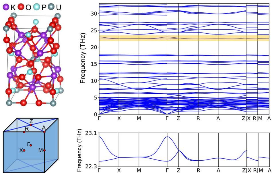
**Figure S22.** The 2NS+WNN phonon of mp-559639  $\text{K}_4\text{UP}_2\text{O}_{10}$  (SG 137), with LOTO.
