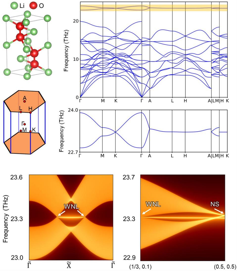
**Figure S25.** The 1NS+WNL phonon of mp-841  $\text{Li}_2\text{O}_2$  (SG 194), with LOTO. The bottom two panels are (100) surface spectra of  $\text{Li}_2\text{O}_2$ . One should notice there only exist WNL-WNL drumhead SSs. The NS cannot serve as termination of SS.
