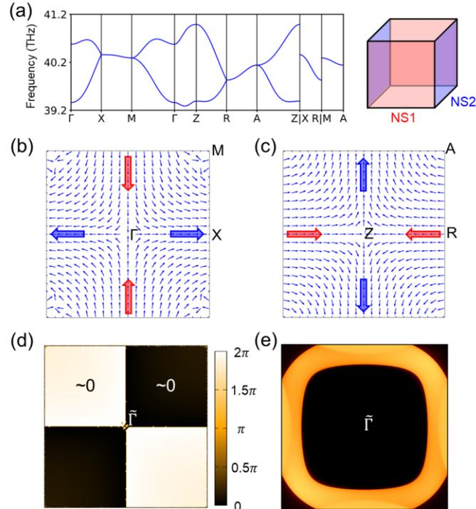
**Figure S8.** (a) The 2NS phonon in bands 29,30 of  $C_4N$ , without LOTO. In-plane Berry curvature  $\Omega_{x,y}(\mathbf{k})$  of band 29 at (b)  $k_z = 0$  and (c)  $k_z = \pi$ . (d) Calculated  $Z(k_x, k_y)$ . (e) The iso-frequency (001) surface contour of  $C_4N$  at 40.0 THz. There exists no SS.
