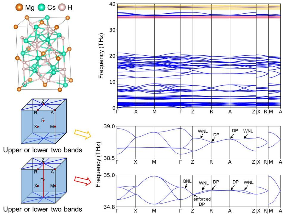
**Figure S32.** The 2NS+WNN and 2NS+HNN phonons in mp-23947  $\text{Cs}_3\text{MgH}_5$  (SG 130), with LOTO.
