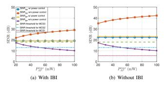
Fig. 8. The impact of power control on the SINRs of simultaneous uplink and downlink transmission.
