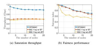
Fig. 7. Performance of the proposed DFDMAC protocol in terms of saturation throughput and accessing fairness.
