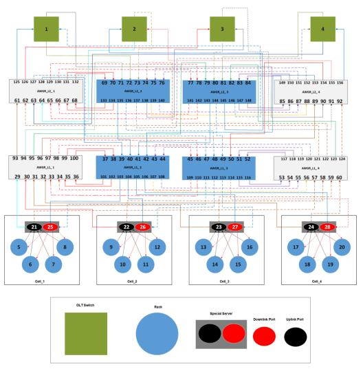
Figure 1.The two tier cascaded AWGRs architecture with four cells.
