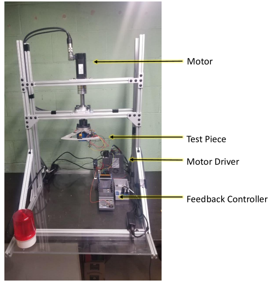
Figure 1: Experimental prototype with one cantilever beam.
