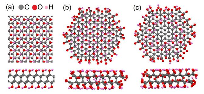
**Figure 4.** Top and side views of the optimized atomic structure of C<sub>2</sub>OH (a), infinite slab (b) unreduced (c) and maximally reduced disc (dot).
