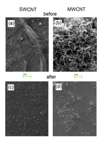
Figure 1. SEM images of SWCNT (a,c) and MWCNT (c,d) before (a,b) and after (c,d) laser treatment.
