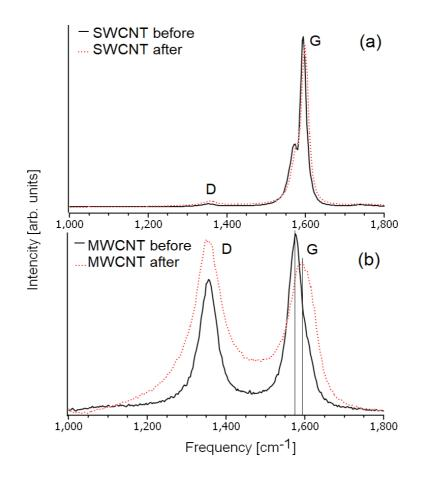
Figure 3. Raman spectra of SWCNT (a) and MWCNT (b) before and after laser treatment.
