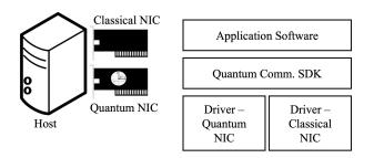
Fig. 6. Hardware and Software for supporting the Abstractions
