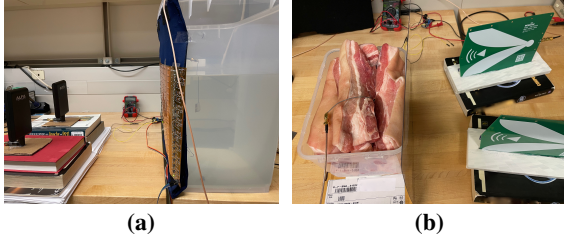
Figure 11: Experiment setups. (a) Water bucket with the surface and fabrics. (b) A box of pork belly with an antenna inside. Both setups have gaps between surface and media.
