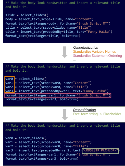
(b) Program normalization performs transforms such as canonicalization and desensitization to avoid spurious discrepancies that prevent matches.
