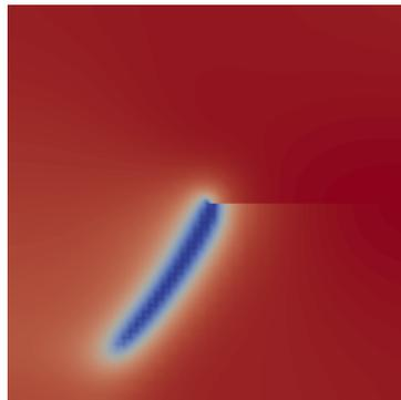
Figure 37: Visualization of the fracture for the SENS test with  $h = 0.022$  after 100 incremental steps with ItE. Red represents the fully intact part of the domain, blue the fully broken part and white stands for the transition zone.
