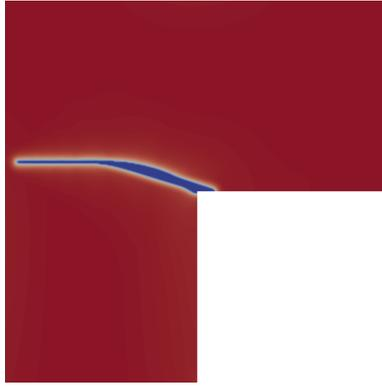
Figure 25: Visualization of the final configuration of the L-shaped panel test with  $h = 1.822$ . Red represents the fully intact part of the domain, blue the fully broken part and white stands for the transition zone.
