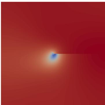
Figure 36: Visualization of the fracture for the SENS test with  $h = 0.022$  after 100 incremental steps with no ItL. Red represents the fully intact part of the domain, blue the fully broken part and white stands for the transition zone.
