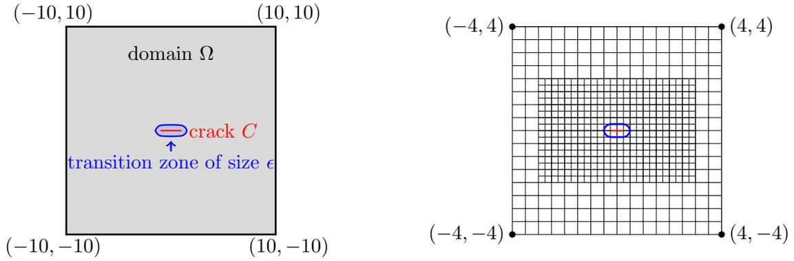
Figure 1: Left: geometry of the two dimensional Sneddon test. Right: zoom-in to the pre-refined crack zone in  $[-4, 4] \times [-4, 4]$  with two global refinement steps and one local refinement step (geometrically pre-refined).
