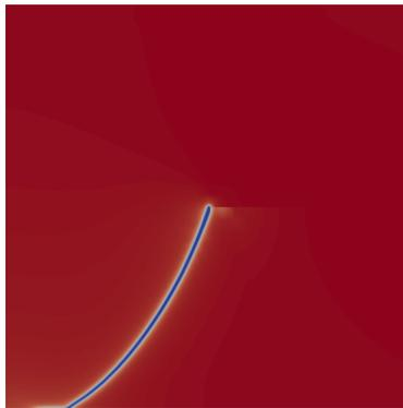
Figure 35: Visualization of the fracture for the SENS test with  $h = 0.0027$  in the final configuration after 135 incremental steps with ItE. Red represents the fully intact part of the domain, blue the fully broken part and white stands for the transition zone.
