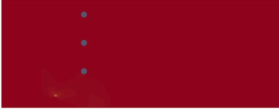
Figure 14: Visualization of the fracture asymmetric three-point bending test with  $h = 0.019$  after 146 incremental steps with ItE. Red represents the fully intact part of the domain, blue the fully broken part and white stands for the transition zone.
