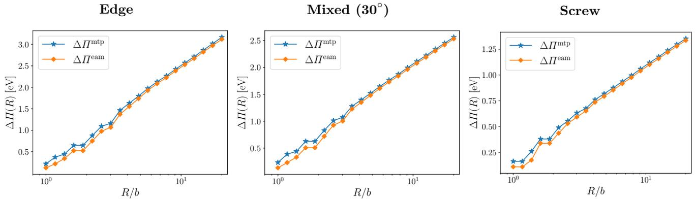
Figure 11: Dislocation energies for the edge, mixed, and screw, dislocation predicted by the MTP and the EAM potential.
