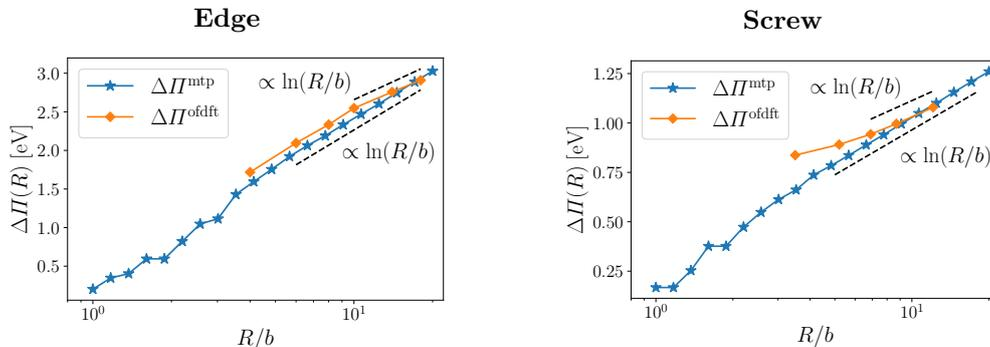
Figure 7: Dislocation energies for the edge and screw dislocation predicted by the MTP and OF-DFT. The agreement between the MTP and OF-DFT is very good and the far-field behavior corresponds to the dislocation energy predicted by linear elasticity (dashed lines) up to some constant core energy.
