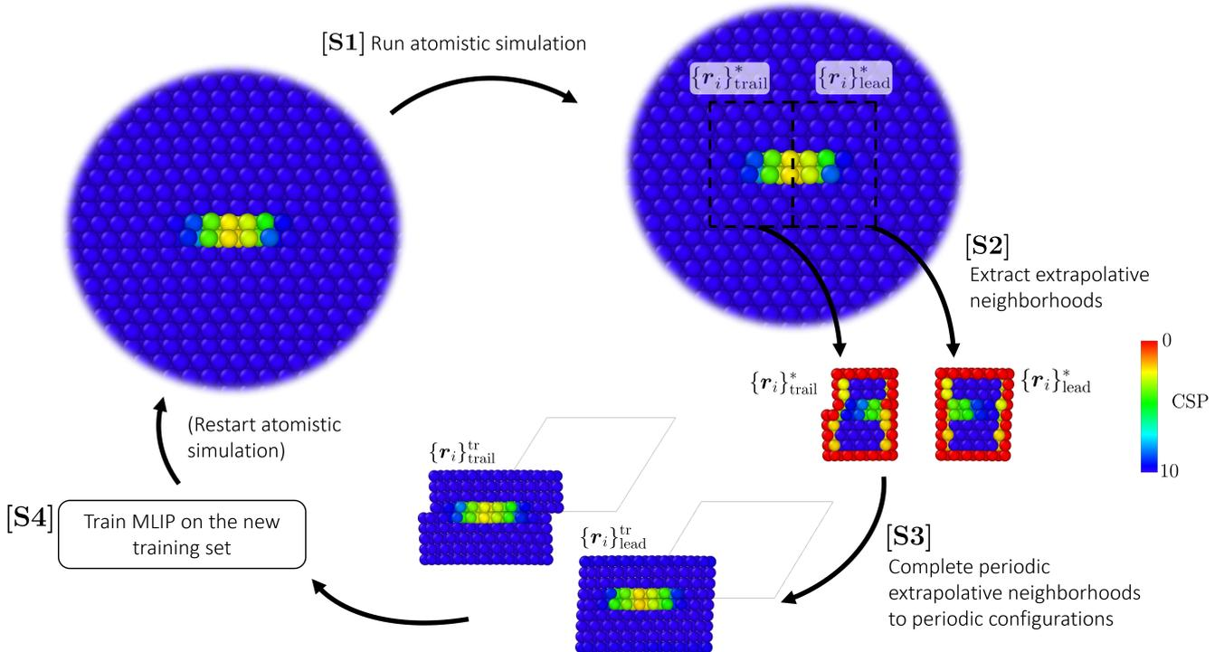
Figure 1: Schematic illustration of the individual steps of the active learning algorithm for fcc dislocations presented in Section 2.2.2. The coloring of the atoms is due to the centrosymmetry parameter (CSP) [51], in order to visualize their deviation from the ideal crystal.
