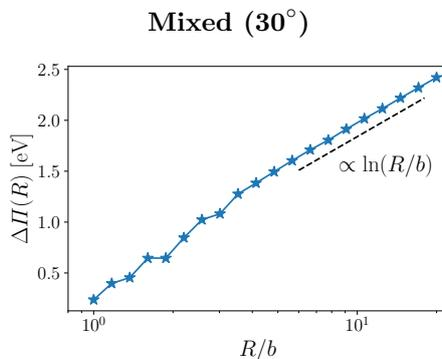
Figure 9: Dislocation energies for the mixed dislocation predicted by the MTP. The far-field behavior corresponds to the dislocation energy predicted by linear elasticity (dashed lines) up to some constant core energy.
