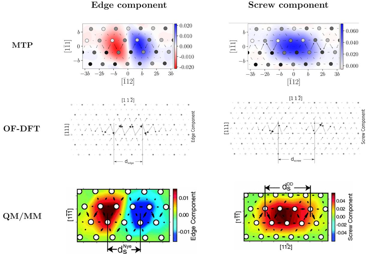
Figure 6: Visualization of the screw dislocation core structure predicted by the MTP, QM/MM [6], and OF-DFT [10], using the edge and screw components of the Nye tensor, and differential displacements. Overall, the agreement between the MTP and DFT core structures is very good, and the splitting distances between the partial dislocations coincide remarkably. The QM/MM and OF-DFT figures are reproduced from [6] and [10] with permission from APS and Elsevier.
