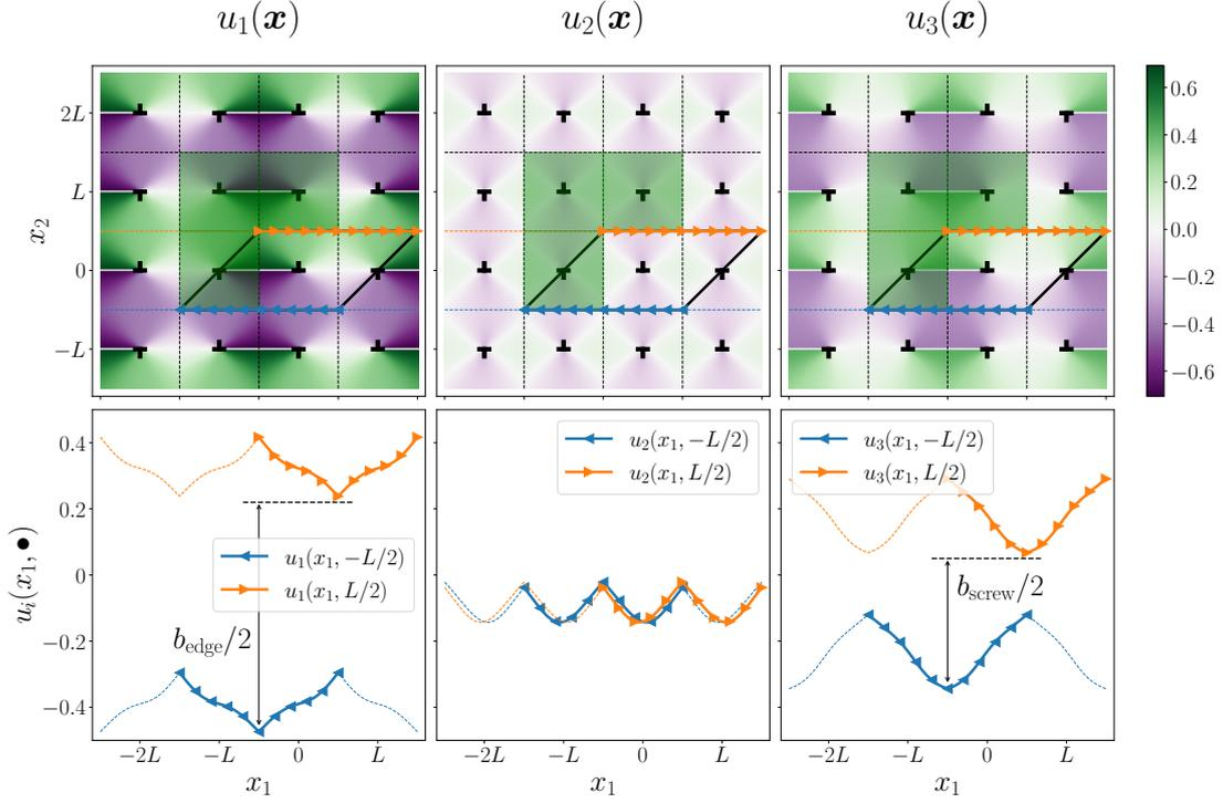
Figure 2: Illustration of the solution (5) that is periodic over a rectangular region containing four linear elastic dislocations. Due to symmetry, the solution is even periodic up to a constant given by half of the magnitude of the Burgers vector over the smaller triclinic cell that contains only two dislocations.
