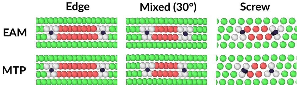
Figure 10: Visualization of the dislocation cores predicted by EAM and MTP using the common neighbor analysis and the DXA.
