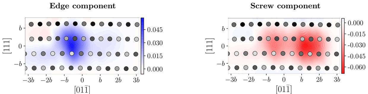
Figure 8: Visualization of the  $30^\circ$ -mixed dislocation core structure predicted by the MTP using the edge and screw components of the Nye tensor.
