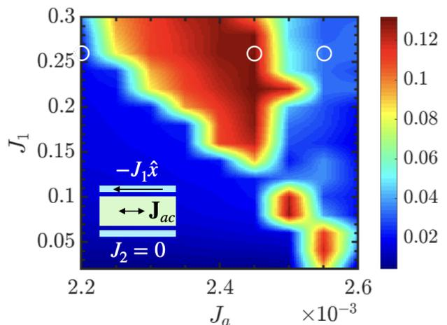
FIG. 2. Phase-diagram displaying the color plot of the output voltage  $V_{DC}$  (in units of  $V_0 = \hbar/2et_{GL}$ ) as a function of  $J_1$  and the amplitude of the AC current (both in units of  $j_0 = \sigma V_0/\xi(0)$ ). We fix  $J_2 = 0$ .
