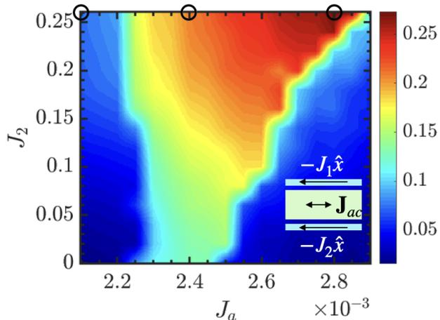
FIG. 6. Phase-diagram displaying the color plot of the output voltage  $V_{DC}$  (in units of  $V_0 = \hbar/2et_{GL}$ ) as a function of  $J_2$  and the amplitude of the AC current (both in units of  $j_0 = \sigma V_0/\xi(0)$ ). We fix  $J_1 = 0.26$ .
