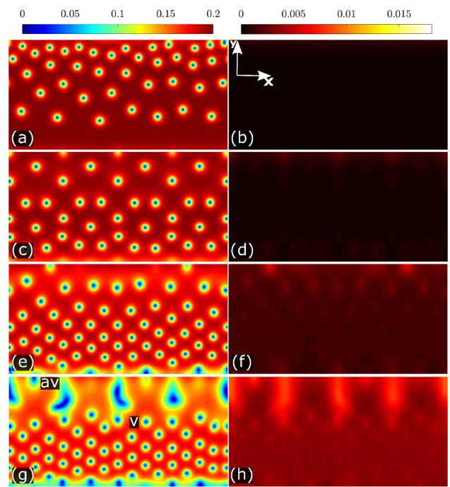
FIG. 5. (Color online) Color plot of the order parameter and local temperature difference  $T - T_0$  at four different times for parameters corresponding to panel (b) in Fig. 3. Each line of the figure corresponds to a black circle in the negative current branch.
