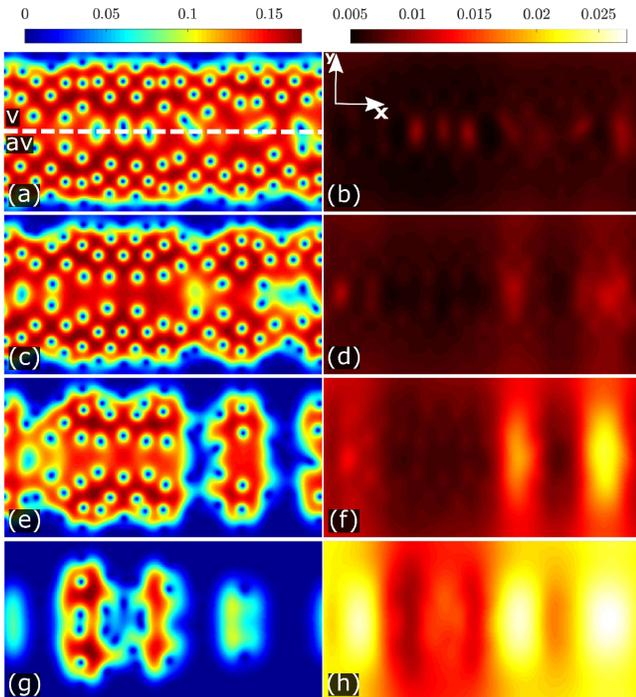
FIG. 8. Evolution of the order parameter (panels in the left column) and the temperature increment  $T - T_0$  (panels in the right column) before the destruction of the superconducting state for parameters of panel (b) in Fig. 7. The white dashed line depicted in panel (a) delineates the superconductor into two distinct halves, with the magnetic flux being composed by vortices in the top region and antivortices in the bottom one.
