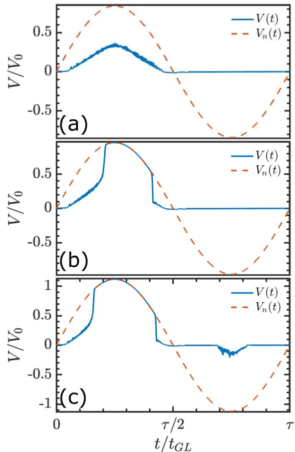
FIG. 7. The voltage signal as a function of time (solid blue line) for  $J_1 = J_2 = 0.26$  and three current values,  $J_a = 2.10 \times 10^{-3}$  (panel (a)),  $J_a = 2.40 \times 10^{-3}$  (panel (b)) and  $J_a = 2.80 \times 10^{-3}$  (panel (c)). In each panel, the red dashed lines represent the voltage if the system was in the normal state.
