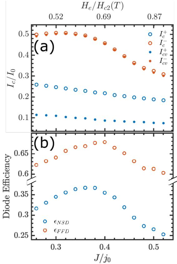
FIG. 13. Panel (a) shows the critical currents  $I_c^+$  (blue circles),  $I_c^-$  (red circles),  $I_{cv}^+$  (blue dots) and  $I_{cv}^-$  (red dots) as a function of the current density in the side stripes  $J$ . Panel (b) shows  $\epsilon_{NSD}$  (blue circles) and  $\epsilon_{FFD}$  (red circles) as a function of  $J$ . Top  $x$  axis relates  $J$  with the value of the inhomogeneous field at the sample edges  $H_e$ .
