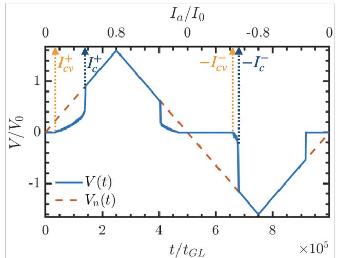
FIG. 9. The voltage signal as a function of time (solid blue line) for a linear current cycle with  $J_1 = J_2 = 0.26$  and total sweep time  $\tau = 10^6 t_{GL}$ . Red dashed curve represents the normal state voltage. The arrows represent the critical currents for the complete destruction of the superconducting state (dark blue) and the onset of vortex motion (orange) at each current polarity.
