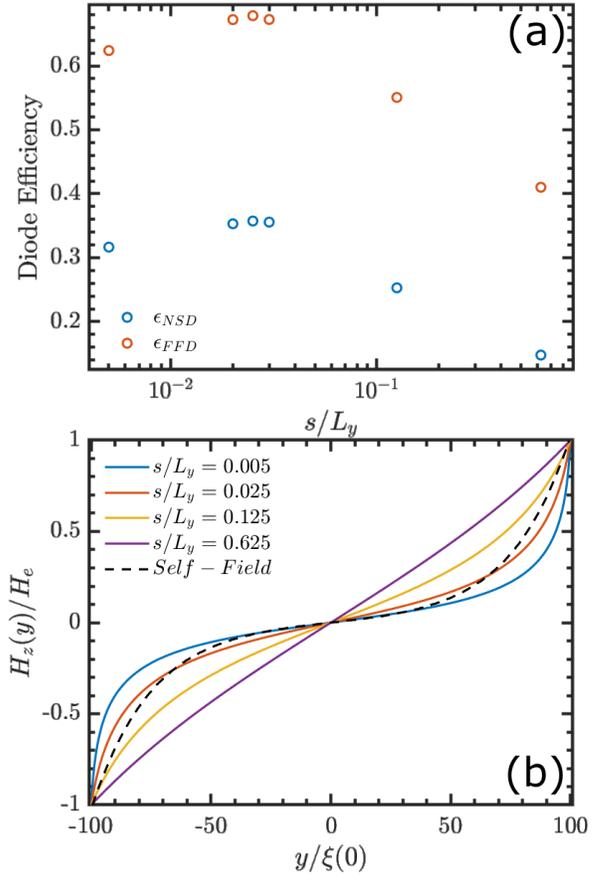
FIG. 14. Panel (a) shows the diode efficiency as a function of the separation between the superconducting film and the lateral wires carrying a current chosen as to induce  $H_e = 0.69H_{c2}(T)$ . Panel (b) presents the inhomogeneous field profile for different values of  $s/L_y$  (solid lines) and the self-field profile of the central superconducting film (black dashed line). All curves are normalized by the field at the edges
