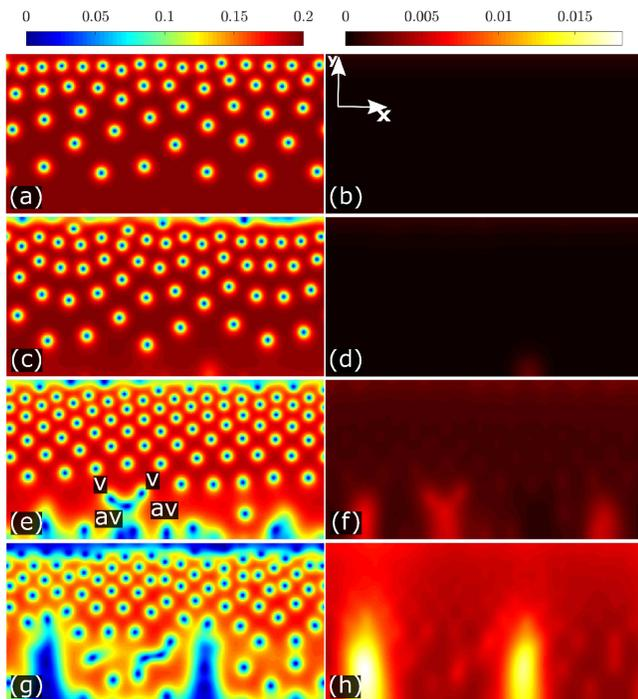
FIG. 4. (Color online) Color plot of the order parameter and local temperature difference  $T - T_0$  at four different times for parameters corresponding to panel (b) in Fig. 3. Each line of the figure corresponds to a black circle in the positive current branch.
