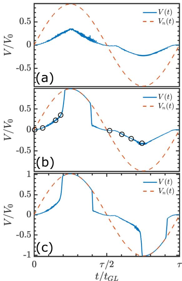
FIG. 3. (Color online) The voltage signal as a function of time (solid blue line) for  $J_1 = 0.26$  and three current values,  $J_a = 2.20 \times 10^{-3}$  (panel (a)),  $J_a = 2.45 \times 10^{-3}$  (panel (b)) and  $J_a = 2.55 \times 10^{-3}$  (panel (c)). In each panel, the red dashed lines represent the voltage if the system were in the normal state.
