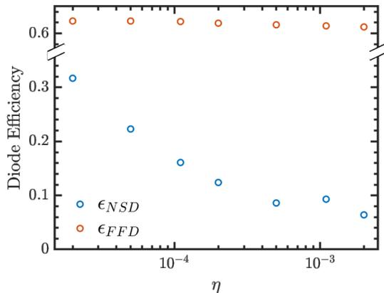
FIG. 11. Efficiencies of the superconducting,  $\epsilon_{NSD}$  (blue circles), and vortex,  $\epsilon_{FFD}$  (red circles), diode effects as a function of the heat transfer coefficient  $\eta$ . Here, we set  $\tau = 10^6 t_{GL}$ .
