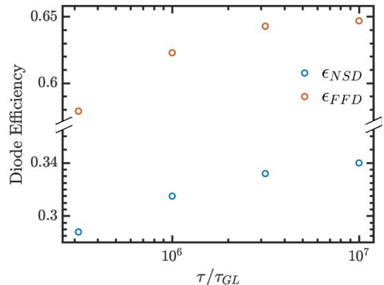
FIG. 12. Efficiencies of the superconducting,  $\epsilon_{NSD}$  (blue circles), and vortex,  $\epsilon_{FFD}$  (red circles), diode effects as a function of total sweep time  $\tau$ . Here,  $\eta = 2 \times 10^{-5}$ .
