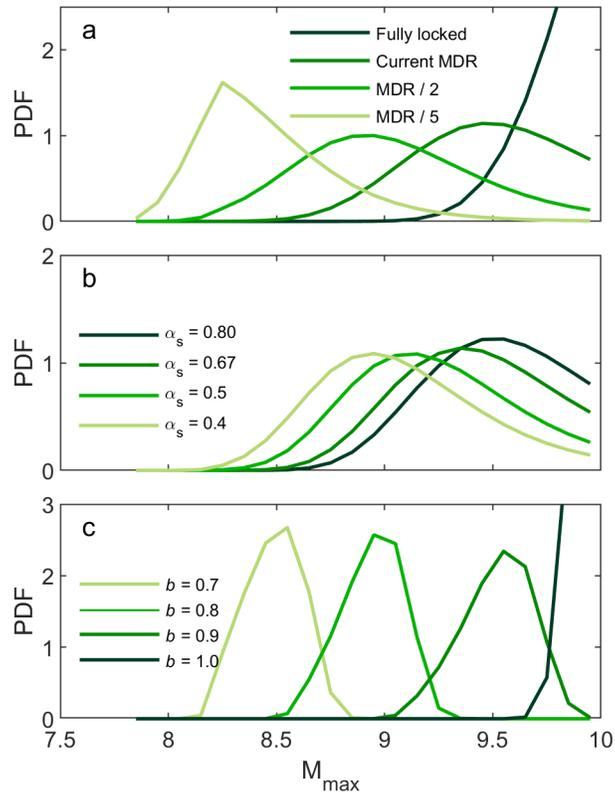
Figure 5: Marginal PDF of  $M_{max}$ ,  $P_{M_{max}}$  for different values of (a) moment deficit rate, (b)  $\alpha_s$ , the proportion of moment released by aftershocks and aseismic afterslip relative to the total moment released, (c)  $b$ -value.
