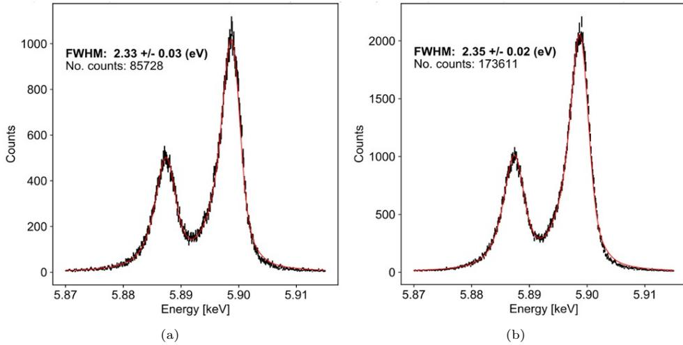
**Fig. 3** Energy spectra from the  $^{55}\text{Fe}$  source collected with the simultaneous operation of the two-channels of the setup, the first with 34-pixel multiplexing (a) and the second with 36-pixel multiplexing (b). Data are represented in black and the best fit is represented in red.
