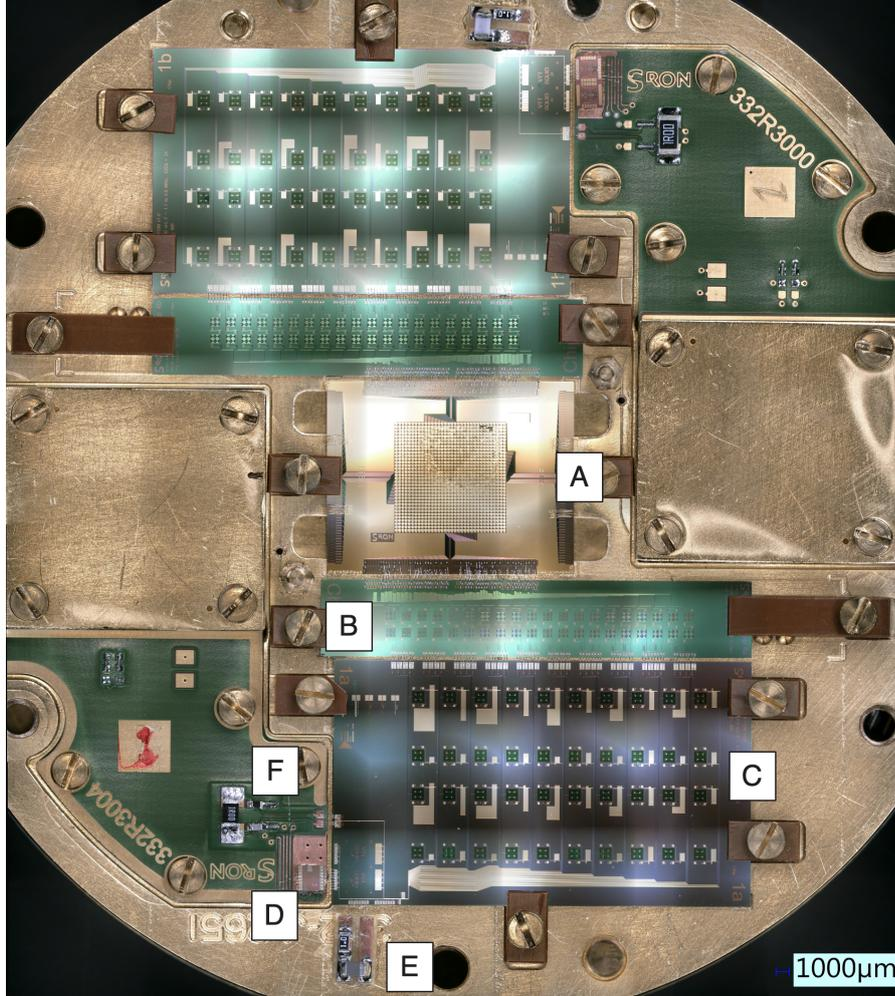
**Fig. 2** Top view of the 50 mK assembly of the setup holding the cryogenic components, with the two populated channels. Visible are the TES array [A], transformer [B] and LC filter [C] chips, the first-stage SQUID [D] with the RC low-pass filter [E] and the bias SMD resistor [F].
