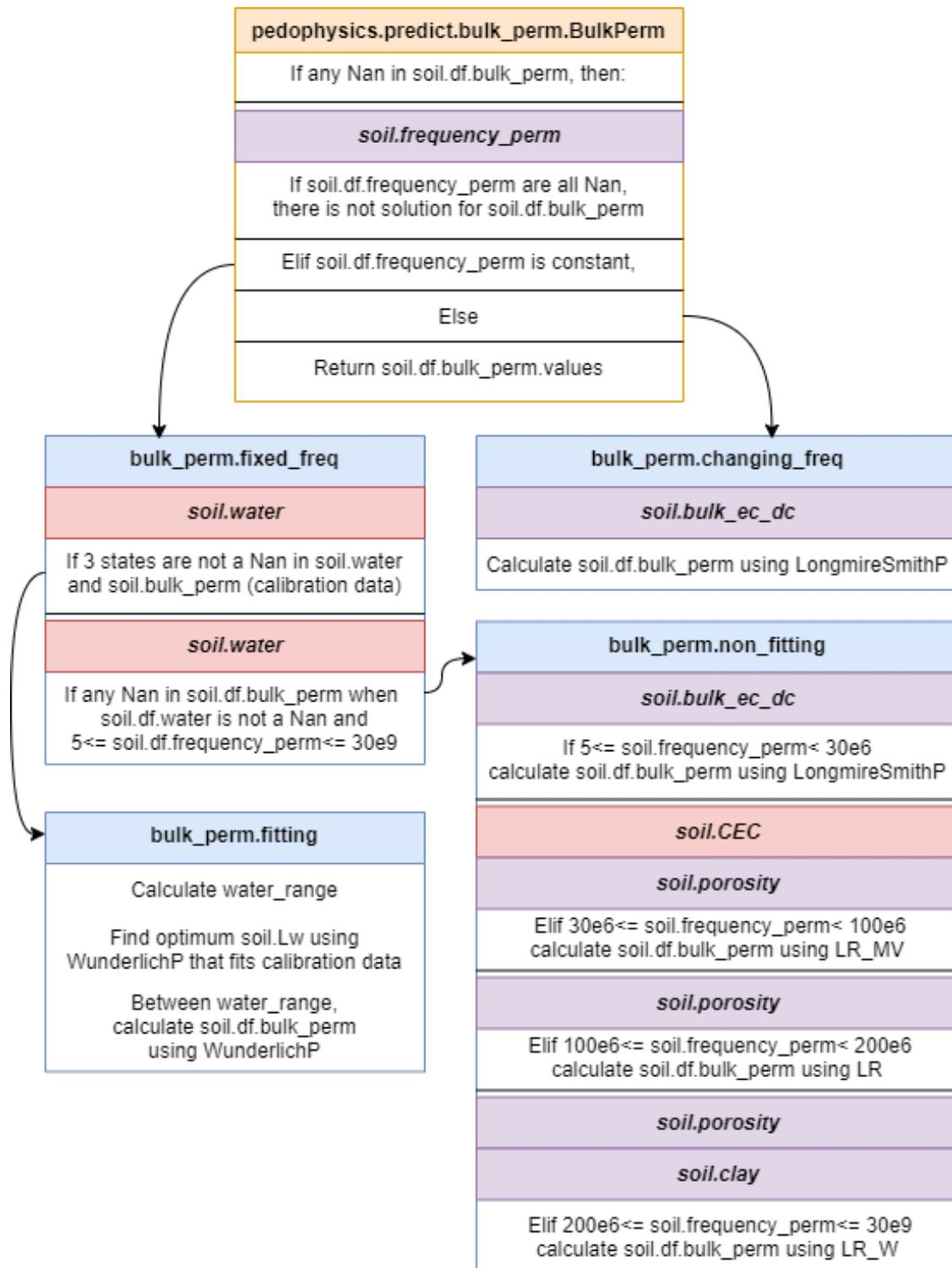
Figure 6. Pedophysics workflow for the calculation of  $\epsilon_b$ . Each block describes a function, which name is at the heading. Light yellow heading is used for the main function `predict.bulk_perm.BulkPerm`, while light blue headings refer to secondary functions. Black horizontal lines divide a block into different conditions. Light red blocks refer to mandatory soil attributes for a condition. Purple blocks refer to mandatory soil attributes that can be derived from other ones.
