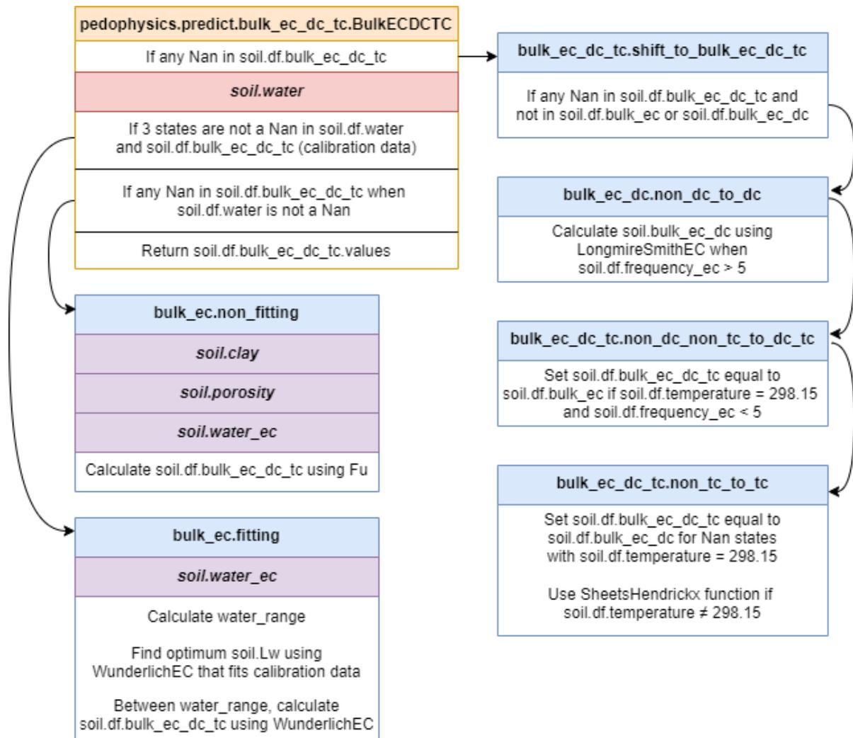
Figure 7 Pedophysics workflow for the calculation of  $\sigma_{dc\_tc}$ . Each block describes a function, which name is at the heading. Light yellow heading is used for the main function `predict.bulk_ec_dc_tc.BulkECDCTC`, while light blue headings refer to secondary functions. Black horizontal lines divide a block into different conditions. Light red blocks refer to mandatory soil attributes for a condition. Purple blocks refer to mandatory soil attributes that can be derived from other ones.
