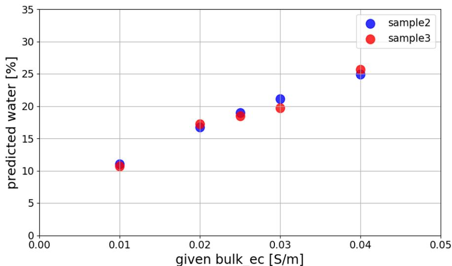
Figure 101 Practical example of a soil with dynamic *Soil.bulk\_ec* and *Soil.clay*, with *Soil.water* as a target. The *Soil* instance 'sample3' has four defined attributes (*Soil.bulk\_ec*, *Soil.clay*, *Soil.porosity*, and *Soil.water\_ec*). The prediction of *Soil.water* is possible because all the required attributes are provided, except for the state 3. The plot (its code is not reproduced here) shows the variation of the given *Soil.bulk\_ec* versus the predicted *Soil.water*.
