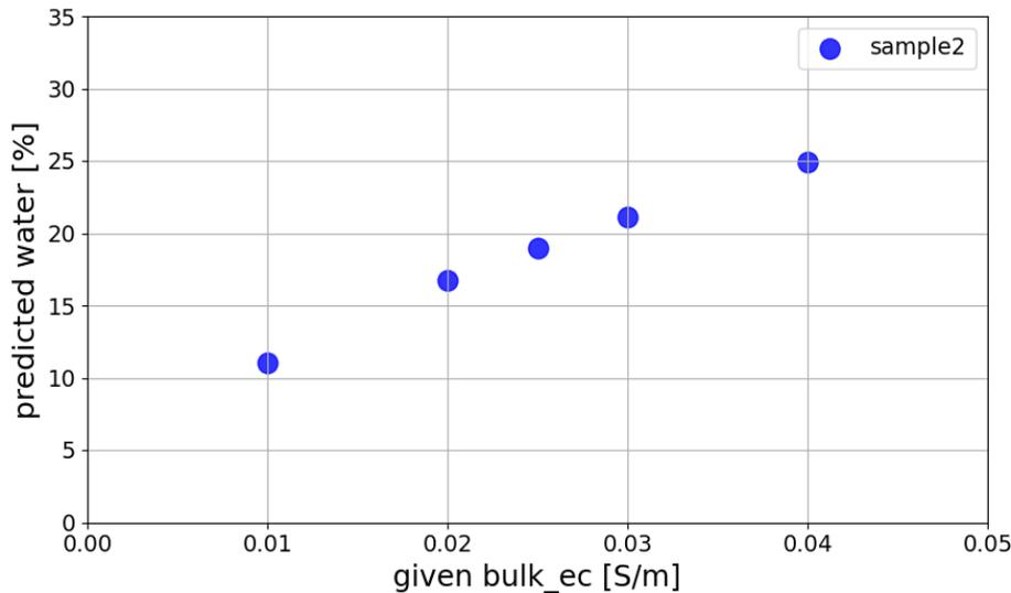
Figure 10 Practical example of a soil with dynamic `Soil.bulk_ec`, and `Soil.water` as a target. The `Soil` instance 'sample2' has four defined attributes (`Soil.bulk_ec`, `Soil.clay`, `Soil.porosity`, and `Soil.water_ec`). The prediction of `Soil.water` is possible because all the required attributes are provided, except for the state 3. The plot (its code is not reproduced here) shows the variation of the given `Soil.bulk_ec` versus the predicted `Soil.water`.
