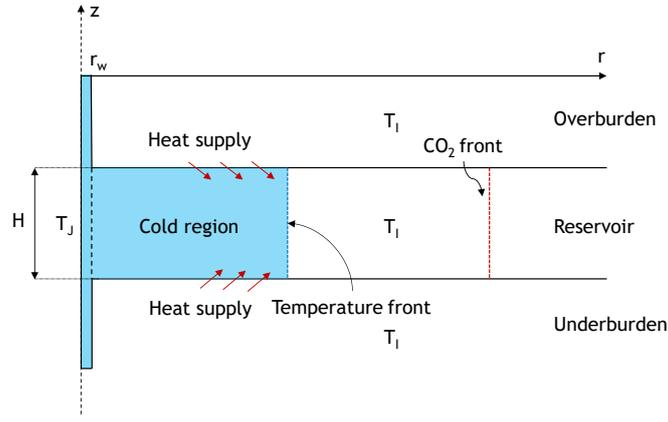
Fig. 3. Schematic of CO<sub>2</sub> injection into a depleted reservoir. The cold part (due to Joule-Thomson cooling effect) is shown in blue.
