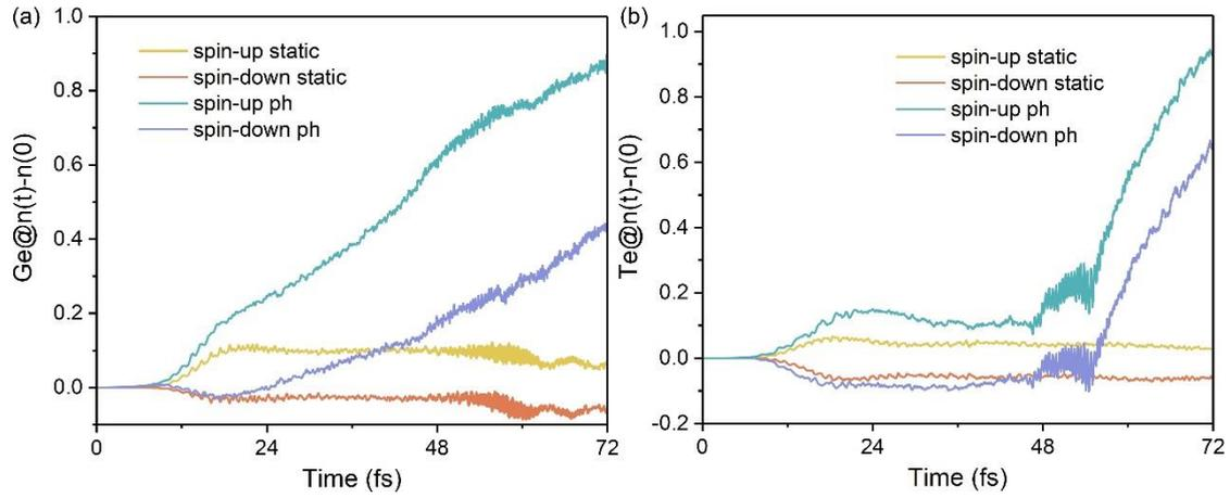
**Figure S4.** Change in the spin-resolved charge ( $\Delta n(t) = n(t) - n(0)$ ) of (a) Ge and (b) Te atom in FGT with (static) and without (ph) nuclear dynamics. Results are shown for pre-excited  $A_{1g}^2$  coherent phonons. The positive (negative) value means the increase (decrease) of electrons.
