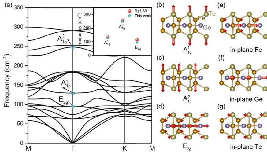
**Figure 1.** (a) Phonon spectra for the Fe<sub>3</sub>GeTe<sub>2</sub> monolayer. The phonon frequency of two  $A_{1g}$  modes and one  $E_{2g}$
