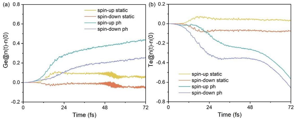
**Figure S5.** Change in the spin-resolved charge ( $\Delta n(t) = n(t) - n(0)$ ) of (a) Ge and (b) Te atom in FGT with (static) and without (ph) nuclear dynamics. Results are shown for pre-excited  $E_{2g}$  coherent phonons. The positive (negative) value means the increase (decrease) of electrons.
