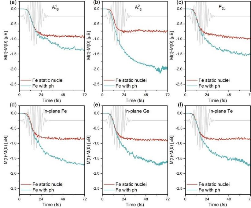
**Figure 2.** Change in the spin moment ( $\Delta M(t)=M(t)-M(0)$ ) dynamics of Fe atom in FGT for full nuclear dynamics (Fe with ph) and in the absence of nuclear dynamics (Fe static nuclei). Results are shown for six pre-excited coherent
