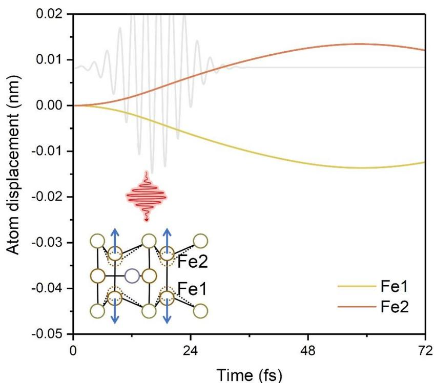
**Figure S1.** The atom displacement of Fe1 and Fe2 atoms in FGT during the pre-excited phonon mode. The linearly polarized laser pulse (gray line) with a photon energy of 1.55 eV, a 12.21 fs FWHM and 11.20 mJ/cm<sup>2</sup> along the out-of-plane direction is applied. The maximum displacement is 0.013 nm with a time period of 60 fs.
