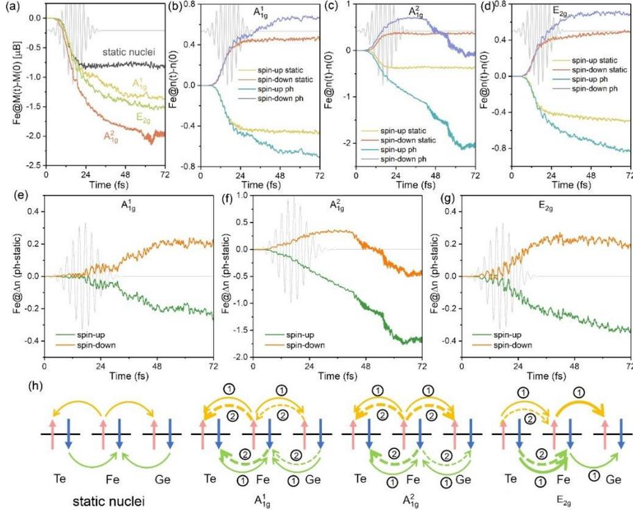
**Figure 3.** (a) Change in the spin moment ( $\Delta M(t)=M(t)-M(0)$ ) dynamics of Fe atom in FGT for full nuclear dynamics
