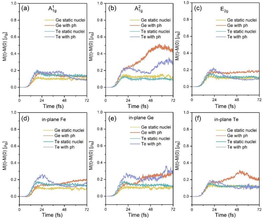
**Figure S2.** Change in the spin moment ( $\Delta M(t)=M(t)-M(0)$ ) dynamics of Ge and Te atoms in FGT for full nuclear dynamics (Ge/Te with ph) and in the absence of nuclear dynamics (Ge/Te static nuclei). Results are shown for six pre-excited coherent phonon modes: (a)  $A_{1g}^1$ , (b)  $A_{1g}^2$ , (c)  $E_{2g}$ , (d) in-plane Fe, (e) in-plane Ge and (f) in-plane Te.
