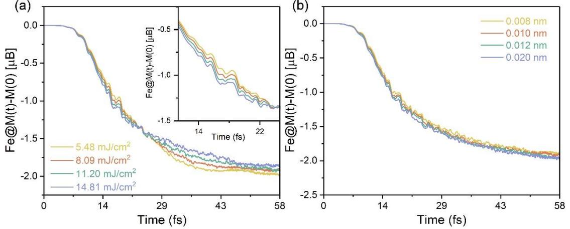
**Figure 5.** Change in the spin moment ( $\Delta M(t)=M(t)-M(0)$ ) dynamics of Fe atom in FGT for full nuclear dynamics with (a) different fluence (FWHM=12.21 fs) and (b) different amplitudes of pre-excited  $A_{1g}^2$  phonon.
