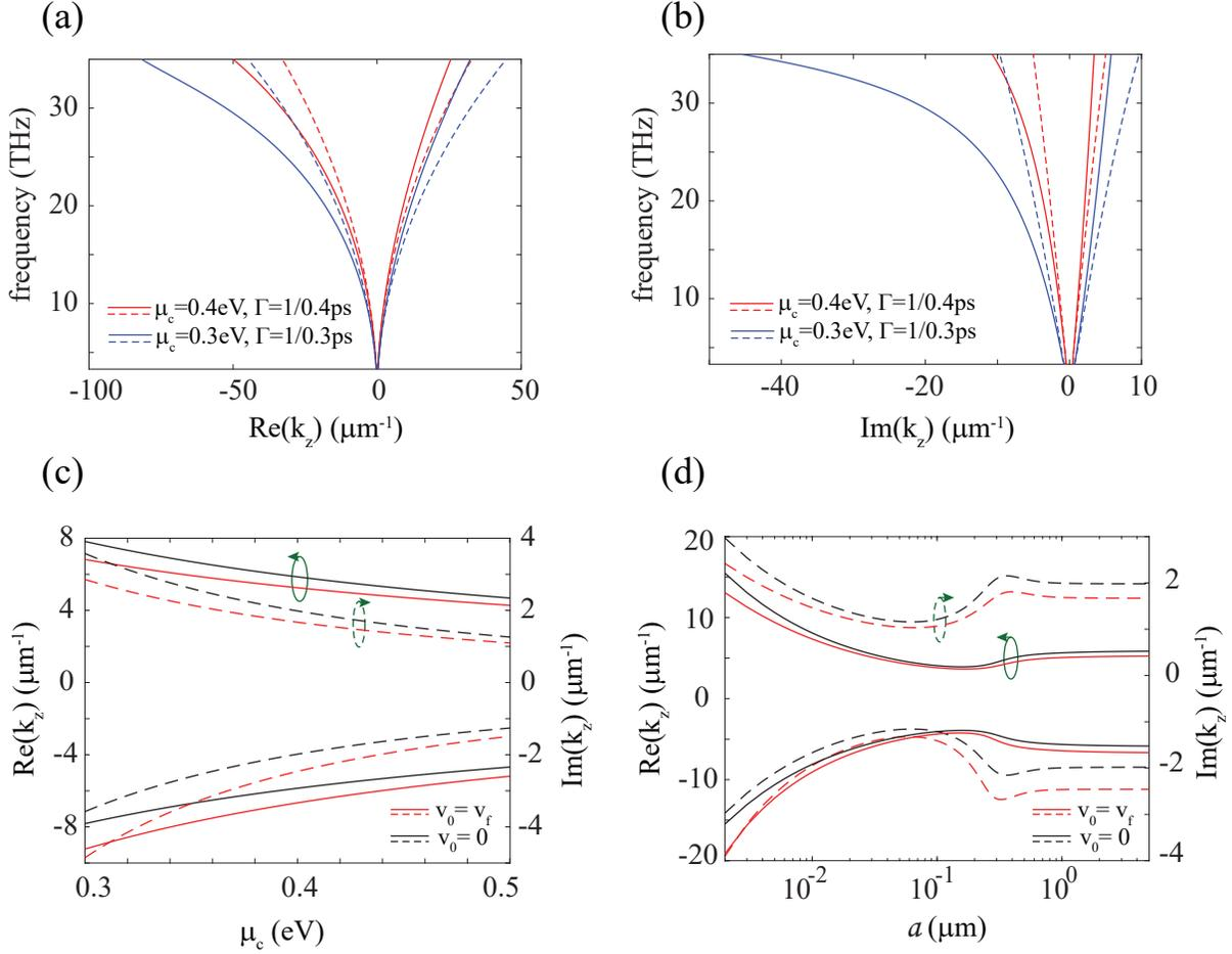
FIG. 2: (a) Real and (b) imaginary parts of wavenumber for biased graphene coating with various scattering rates, here we assume  $k_z = Re(k_z) - iIm(k_z)$ . Solid and dashed lines represent the biased ( $v_0 = v_f$ ) and unbiased ( $v_0 = 0$ ) cases, respectively. Real and imaginary part of wavenumber of the *SPP* mode at  $f = 15$  THz versus (c) chemical potential and (d) the radius of the fiber for  $v_0 = v_f$  and  $v_0 = 0$ .
