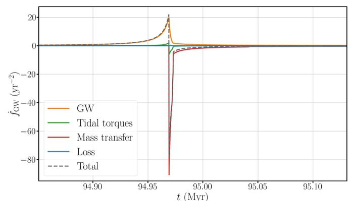
**Fig. 2.** Break-up of the contributions to  $\dot{f}_{\text{GW}}$  from the different terms in Eq. (16) for the system shown in Fig. 1, zoomed around the moment mass transfer begins. We have combined the donor and accretor contributions into a single term for the mass-transfer and for the tidal torque term.
