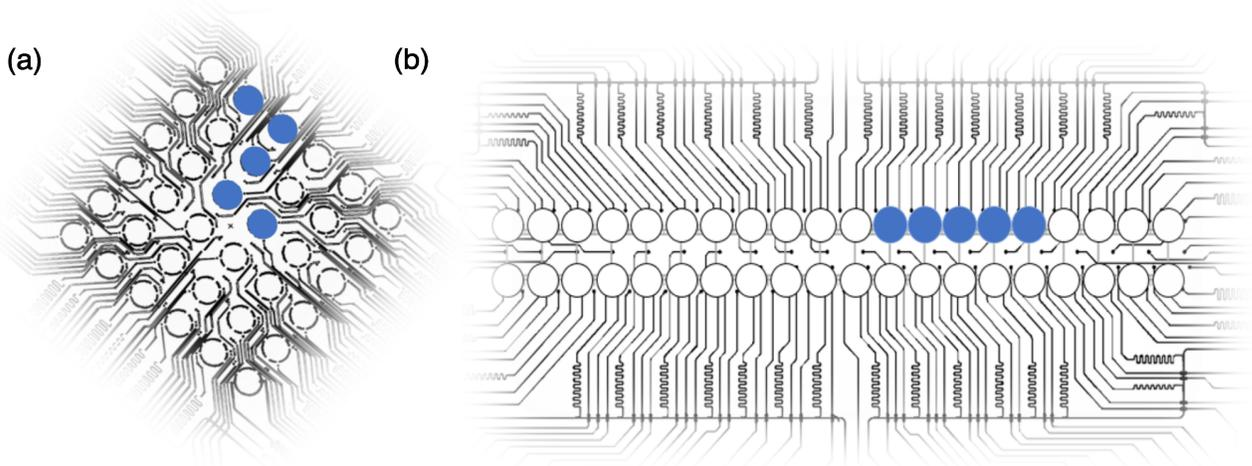
Figure S1. **Schematics of processor I (a) and processor II (b).** Processor I has a  $6 \times 6$  qubit array, and processor II has a  $2 \times 20$  qubit ladder. All qubits used in the experiment are depicted with blue filled circles.
