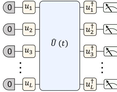
Figure S2. **Pulse sequence for probing the SFF and pSFF dynamics with a randomized measurement protocol.** We start with an initial product state  $|0\rangle^{\otimes L}$ . Before and after the unitary time evolutions  $\hat{U}(t)$  of the Floquet or the Hamiltonian models, we apply random Clifford gates and their inverses, respectively. Finally, we measure all qubit simultaneously for  $2^L$  occupation probabilities.
