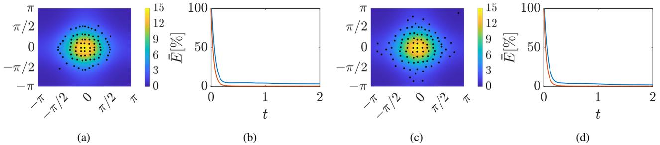
Fig. 2: Robustness to limited sensing ( $K_p = 100$ , (a, b)  $\Delta = 0.1\pi$ , (c, d)  $\Delta = \pi$ ). (a, c) Final displacement of the system on top of the desired density; (b, d) time evolution of the percentage error for the discrete (blue) and continuous case (orange).
