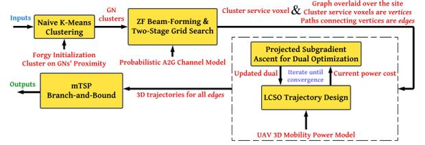
Fig. 3: The solution flow of our cross-layer optimization approach.
