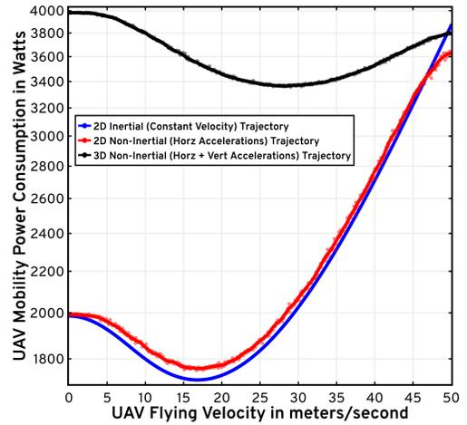
Fig. 2: UAV power analyses for 2D inertial trajectory (blue), 2D non-inertial trajectory (horizontal accelerations) where its average velocity is equal to the abscissa (red), and 3D non-inertial trajectory (horizontal and vertical accelerations) where its average velocity is equal to the abscissa (black).
