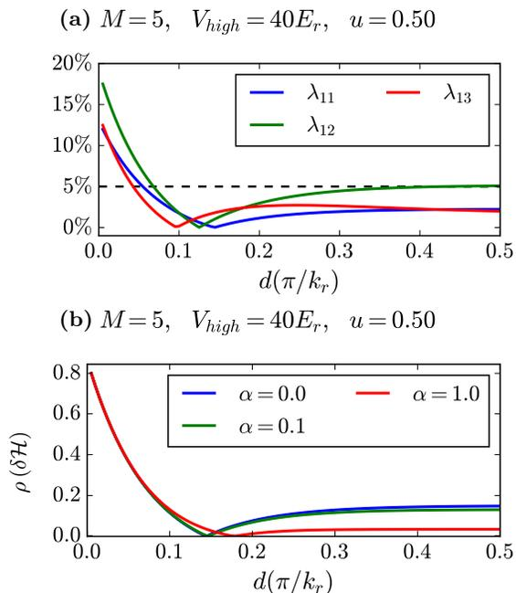
FIG. 6. (a) The elements  $\lambda_{11}, \lambda_{12}$  and  $\lambda_{13}$  versus the length of the linearly extended boundary  $d$  and  $\alpha = 0$ . (b) The spectral radius of the matrix  $\delta\mathcal{H}$  versus the length of the linearly extended boundary  $d$  and three cases of the slope  $\alpha = 0, 0.1, 1$  in units of  $E_r \cdot k_r$ .
