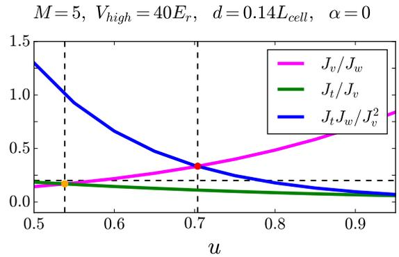
FIG. 9. The ratios  $J_v/J_w$ ,  $J_t/J_v$  and  $(J_t/J_v)/(J_v/J_w)$  for the hopping amplitudes of a system with  $M = 5$ ,  $V_{high} = 40E_r$  and  $d = d_{crit}$ . The horizontal dashed line shows the 0.2 ratio value, while the vertical dashed lines show the values of  $u$  where the crossing of  $J_v/J_w$  with  $J_t/J_v$  and  $(J_t/J_v)/(J_v/J_w)$  occurs.
