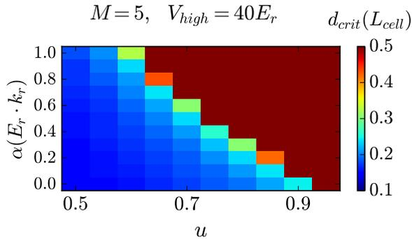
FIG. 8. Color plot of the  $d_{crit}$  in units of  $L_{cell}$  defined as the point of minimum of the spectral radius versus the ratio of the heights of the potential barriers  $u$  and the slope  $\alpha$ . The area colored in deep red indicates the parameter region where the spectral radius has no minimum.
