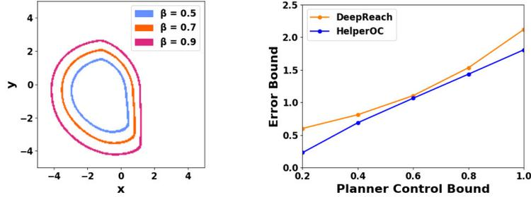
Figure 2: (Left) TEB for system (6) with different planner control bounds  $\beta$ . Training parameters: 40k pre-train iterations, followed by 110k training iterations. The model is trained until convergence. Total training took 10h32m on a NVIDIA A30. As  $\beta$  increases, the TEB grows larger. (Right) comparison between standard dynamic programming based HJ reachability (using codebase HelperOC) and DeepReach. Empirically, DeepReach produces more conservative error bounds.
