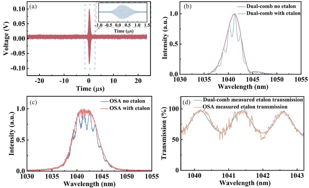
Fig. 5. (a) Single-shot interferogram (inset: zoom-in of the interferogram in the blue box portion). (b) Comparison of the spectrum with and without etalon measured with dual-comb spectroscopy. (c) Comparison of the spectrum with and without etalon measured with the OSA. (d) Comparison of the etalon transmission spectrum measured with the dual-comb system and OSA.
