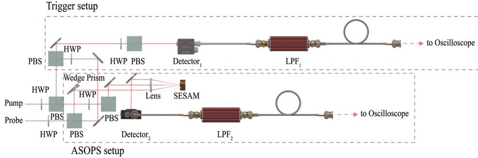
Fig. 6. Setup of the ASOPS-based SESAM measurement. HWP, halfwave plates; PBS, polarizing beamsplitter; LPF, low-pass filter.
