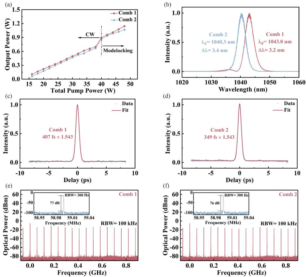
Fig. 2. The performance evaluation of the dual-comb. (a) Laser output power versus total pump power, (b) Optical spectra of comb 1 (blue) and comb 2 (red), (c)-(d) Autocorrelation trace with  $\text{sech}^2$  fit, (e)-(f) Laser output detected by a fast photodiode and measured by an electrical spectrum analyzer where the insets indicate signal-to-noise ratio with a resolution bandwidth (RBW) of 300 Hz.
