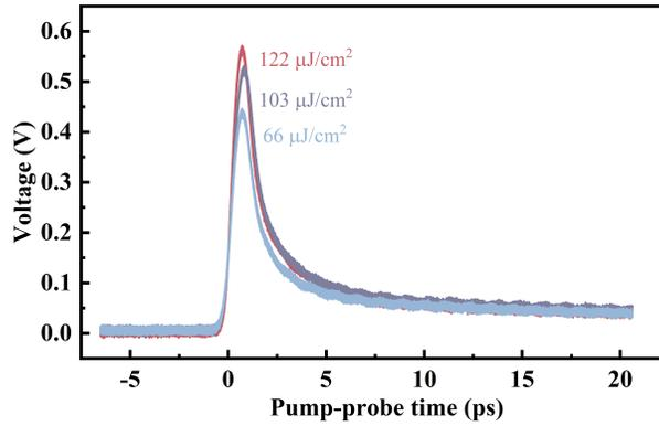
Fig. 7. ASOPS-based SESAM measurement at different pump fluences.
