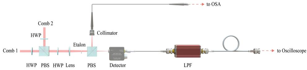
Fig. 4. Interferogram measurement setup. HWP, halfwave plate; PBS, polarizing beamsplitter; LPF, low-pass filter; OSA, optical spectrum analyzer.
