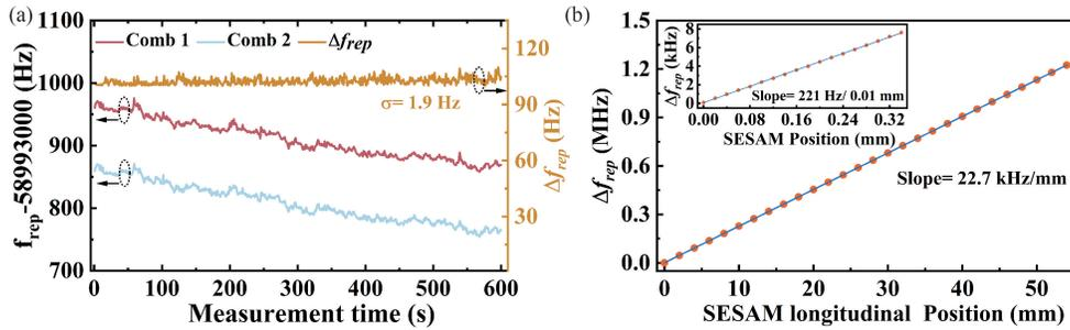
Fig. 3. (a) Temporal evolution of the repetition rates and their difference. (b) Repetition rate difference versus the SESAM longitudinal position.
