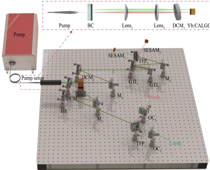
Fig. 1. Schematic drawing of the dual-comb laser system. SESAM, semiconductor saturable absorber mirror; TFP, thin-film polarizer; DCM, dichroic mirror; HR, high reflection; M, mirror; OC, output coupler; GTI, Gires–Tournois interferometer .
