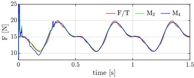
Fig. 5. Comparison of the registered forces (F/T in red) against the estimated ones ( $M_2$  in green and  $M_4$ ) without the use of the sensor.
