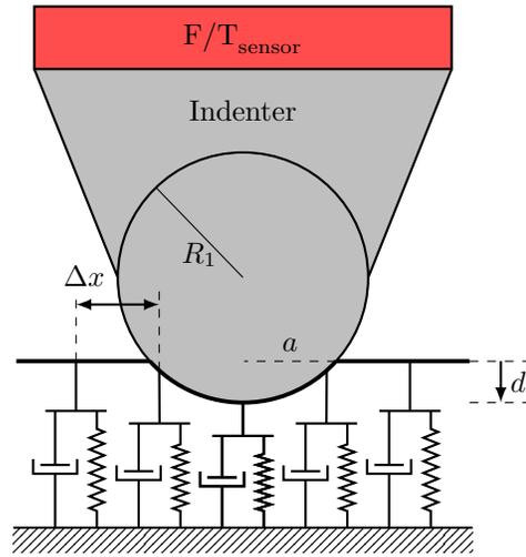
Fig. 1. Schematic of a spherical indenter in constant with a viscoelastic half-plane.  $\Delta x$  is the distance between the viscous elements,  $a$  represents half of the projection of the circle's portion in contact,  $d$  is the maximum penetration and  $R_1$  is the equivalent radius of the sphere in the viscoelastic half-plane.
